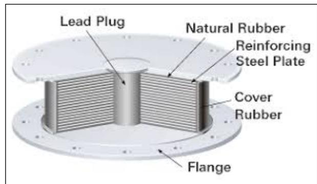
Figure 1: Lead Plug Bearing
