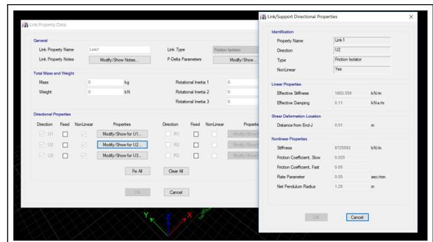
Figure 7: Friction Pendulum Bearing Properties Assigned to the Building
