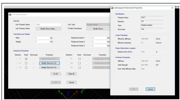
Figure 6: Lead Plug Bearing Properties Assigned to the Building
