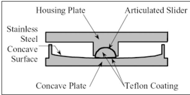
Figure 2: Friction Bearing
