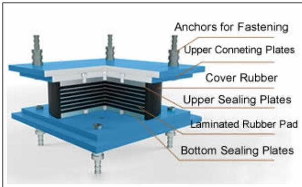
Figure 3: High Damping Rubber Bearing
