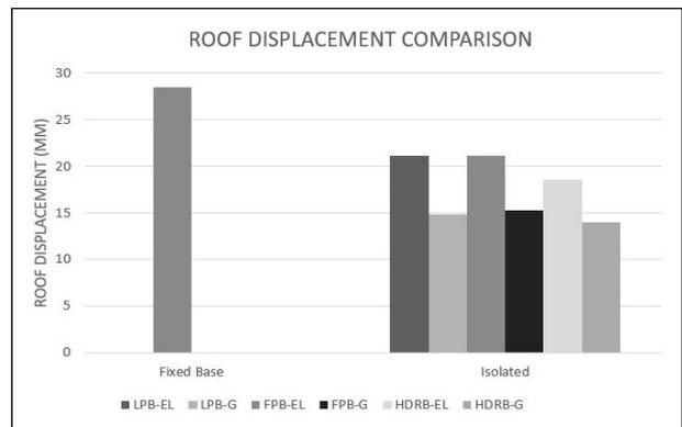
Figure 13: Comparison of Relative Roof Displacement
