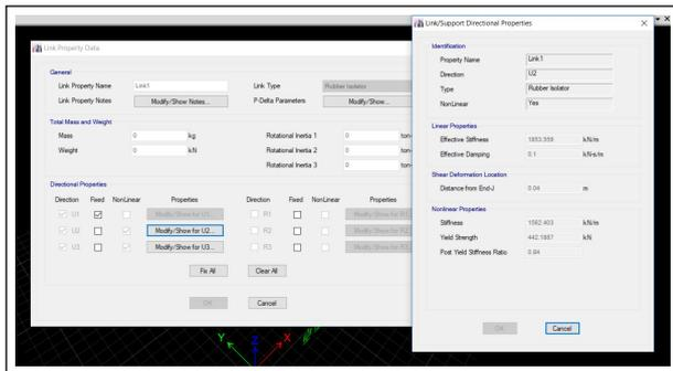
Figure 5: Lead Plug Bearing Properties Assigned to the Building
