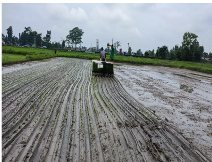
Figure 2: Float type mechanical rice transplanter in operation
