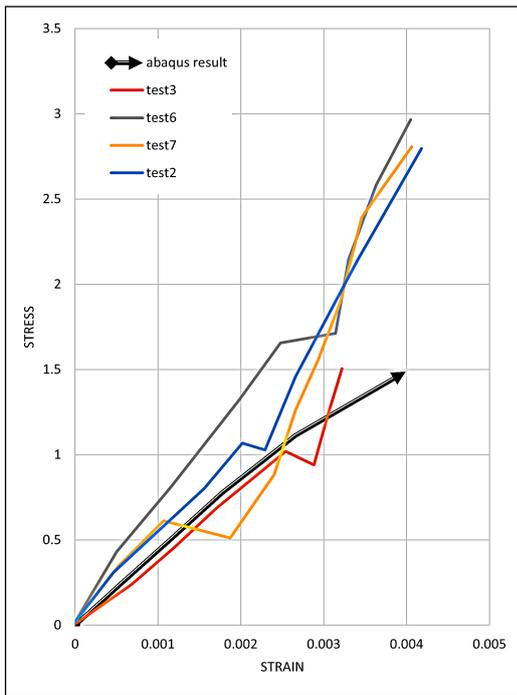
Figure 4: Comparison of Stress-Strain Diagram of Test results to Numerical model
