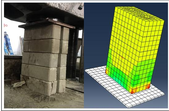
Figure 3: Failure of Masonry Prism (Experimental and Numerical Visualization)
