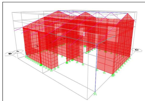
Figure 5: Macro-modelling of whole building in SAP 2000 V22.0.0
