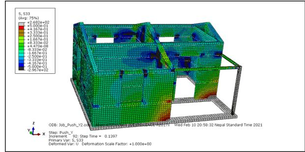
Figure 12: Stress in various components of building during push over analysis
