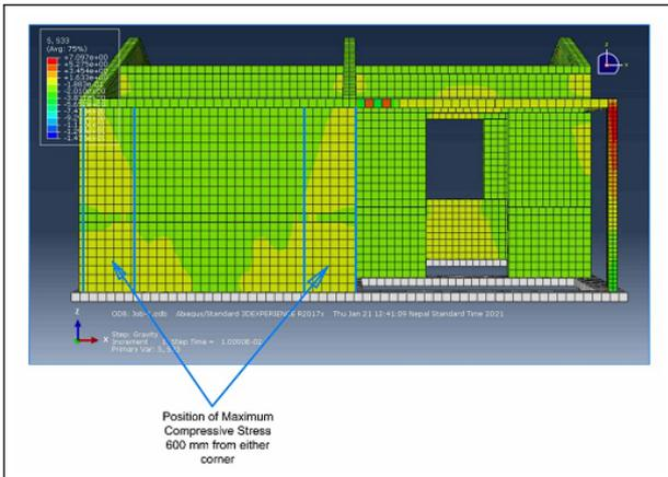
Figure 11: Stress around solid wall corners
