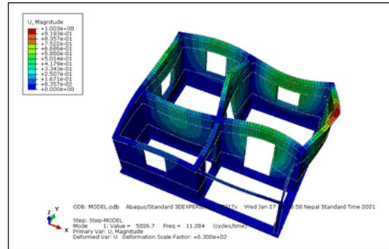
**Figure 7:** Fundamental mode shape of building: Frequency 11.294 Hz.
