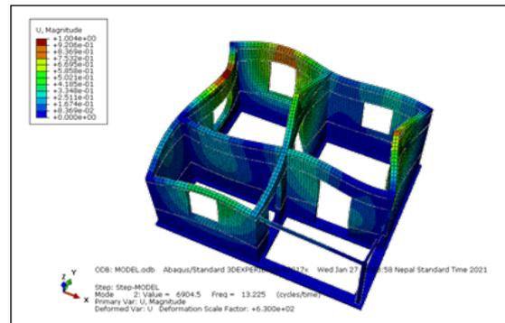
**Figure 8:** Second mode shape of building: Frequency 13.225 Hz.
