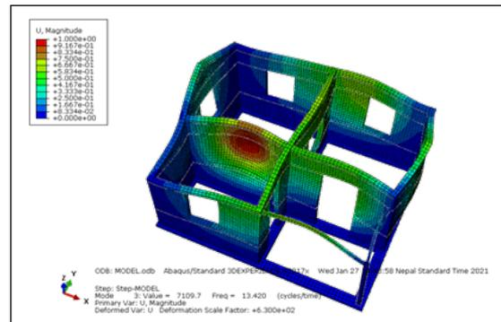
**Figure 9:** Third mode shape of building: Frequency 13.420 Hz.
