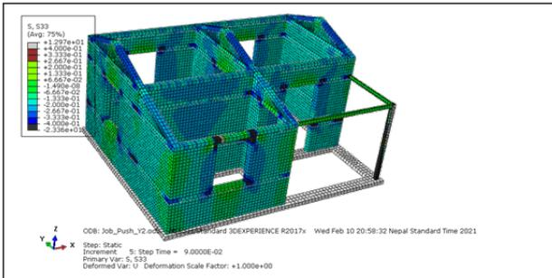
Figure 10: Stress in various components of building with Dead load + Imposed load
