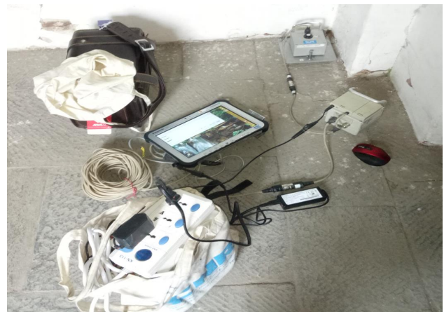
Figure 2: Instrument setup with Base plate, PIC sensor, Transducer, Inverter, Battery and laptop all connected with wire
