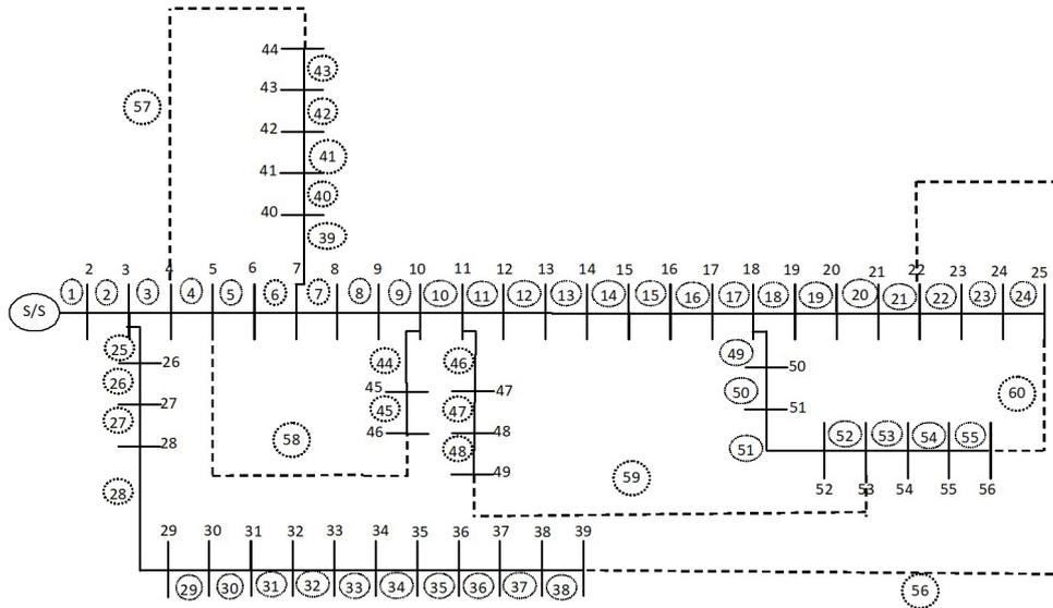
**Figure 7: NEA-56 Bus Radial Distribution System**
