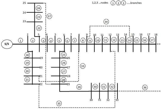
**Figure 5:** IEEE-33 Bus Radial Distribution System
