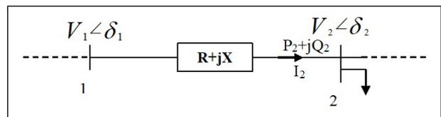
**Figure 1:** Simple Radial Distribution System
