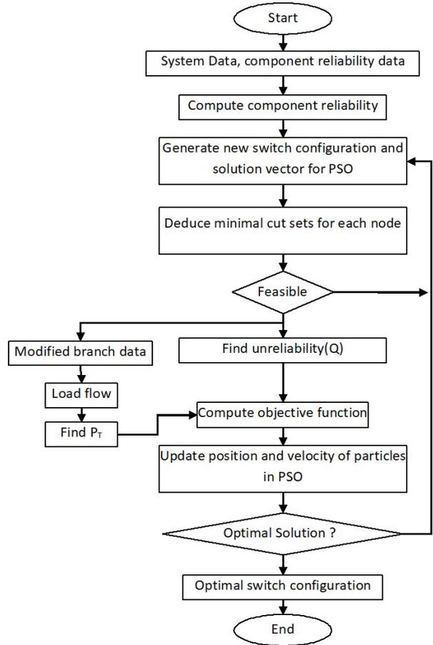
**Figure 4:** Flowchart showing Overall Procedure for Network Reconfiguration
