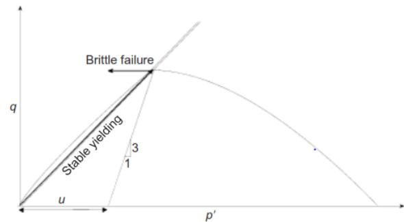
Figure 4: Stress path during plastic limit test
