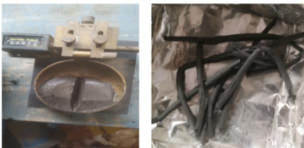
**Figure 2:** Liquid Limit and Plastic Limit Test
