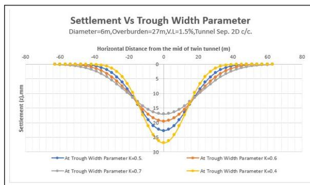
**Figure 13: Settlement Vs Troughwidth Parameter**
