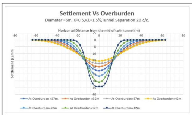
**Figure 12: Settlement Vs Overburden Plot**
