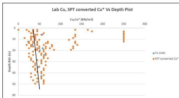
**Figure 3:** Lab Cu and SPT converted Cu plot.
