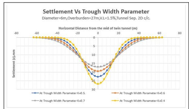
**Figure 13: Settlement Vs Troughwidth Parameter**
