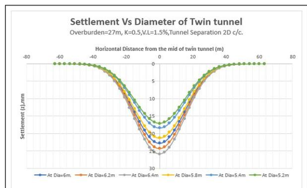
Figure 11: Settlement Vs Diameter Plot
