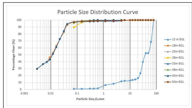
**Figure 9:** Particle Size Distribution of Lagankhel Intermediate Station for TBM selection
