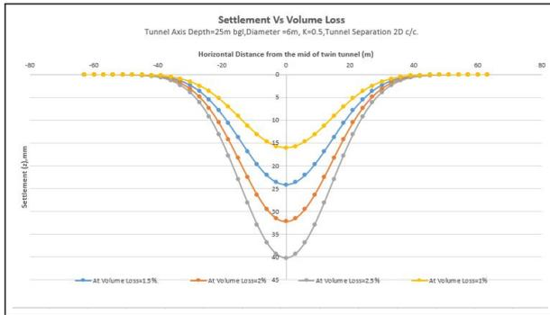
Figure 14: Settlement Vs Volume Loss
