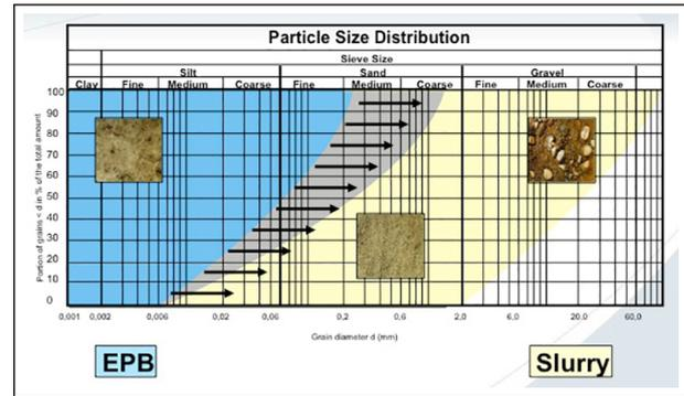
**Figure 8:** TBM selection criteria as per Herrenect TBM Company
