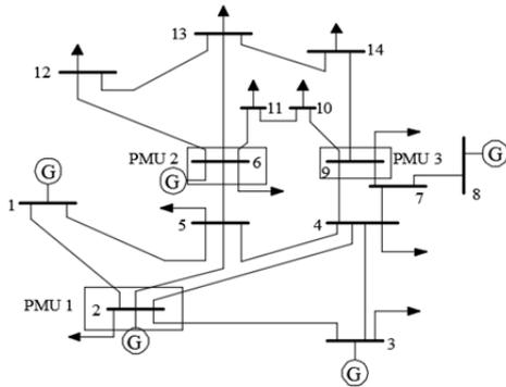
**Figure 3:** Optimal PMU Placement in IEEE-14 Bus Test System
