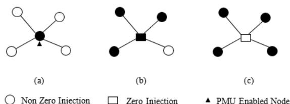
**Figure 1:** Topological observability rules based on PMU
