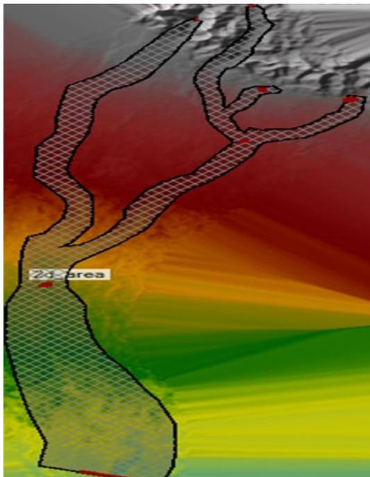
**Figure 3:** 2-D geometric data created in RAS Mapper
