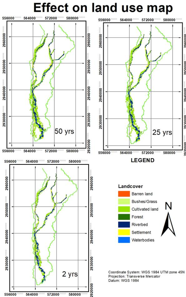
**Figure 5:** Effect of flooding on various land use in Ratuwa Khola
