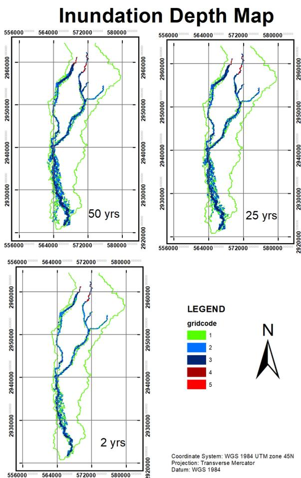
**Figure 4:** Inundation depth map of various return period
