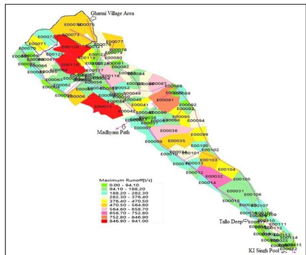
**Figure 7:** Maximum runoff for each sub-catchments
