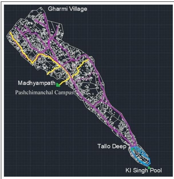
**Figure 8:** Drainage network with free outfall at three locations of Lamachaur catchment
