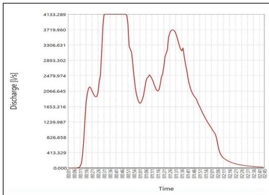
**Figure 11:** Time history of simulated discharge for conduit no. 3010036
