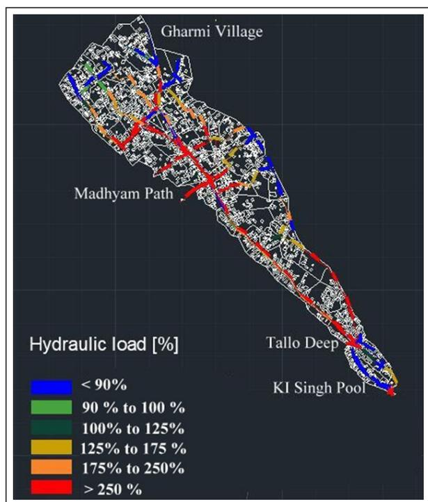
**Figure 15:** Hydraulic load capacity of entire network system for average rainfall intensity of 323 l/s-ha
