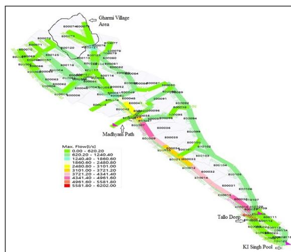
Figure 9: Maximum discharge in the entire network system
