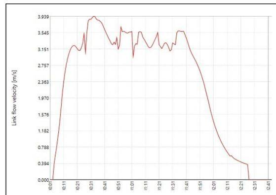
**Figure 14:** Time history of maximum velocity for conduit no. 3010013 (time in x-axis)
