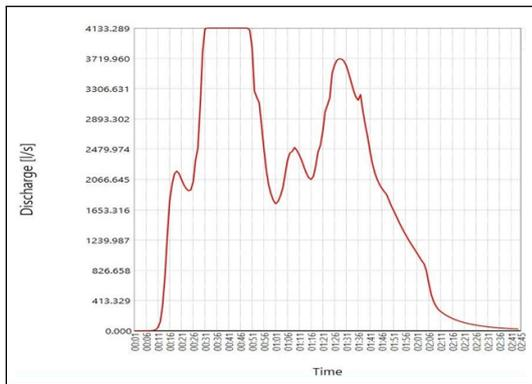
**Figure 11:** Time history of simulated discharge for conduit no. 3010036
