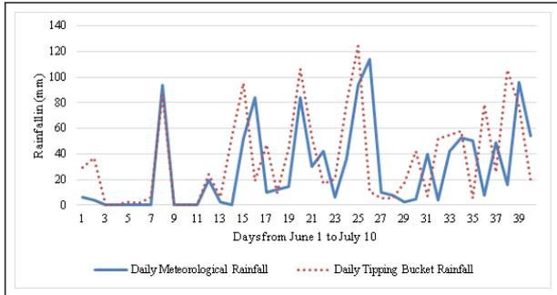
**Figure 4:** Comparison of daily rainfall data obtained from meteorological station with tipping bucket rainfall data
