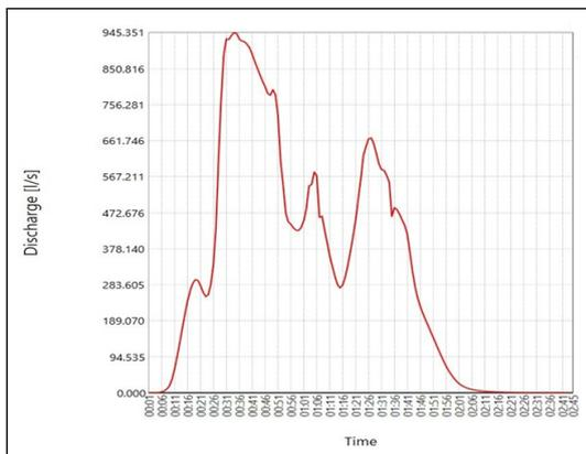
**Figure 12:** Time history of simulated discharge for conduit no. 3010013
