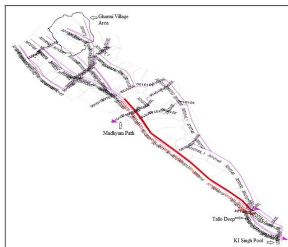
Figure 10: Location of maximum discharge greater than 2.5m<sup>3</sup>/sec for rainfall event of September 9, 2018
