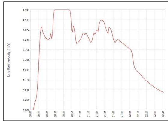
**Figure 13:** Time history of maximum velocity for conduit no. 3010036 (time in x-axis)
