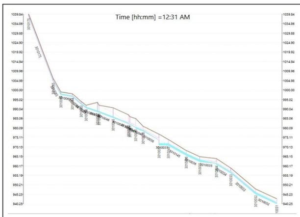
**Figure 17:** Analysis of simulation of rainfall event for existing network
