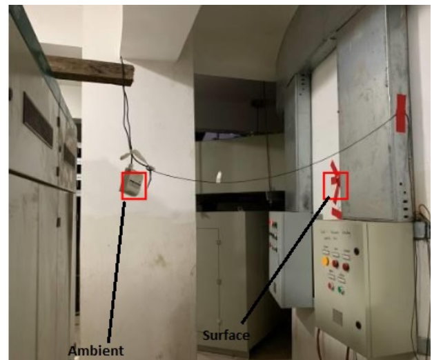
Figure 5: Surface and ambient temperature thermometer placement at upper surface
