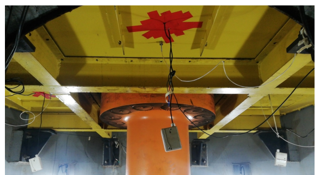
Figure 6: Surface and ambient temperature thermometer placement at lower cover surface
