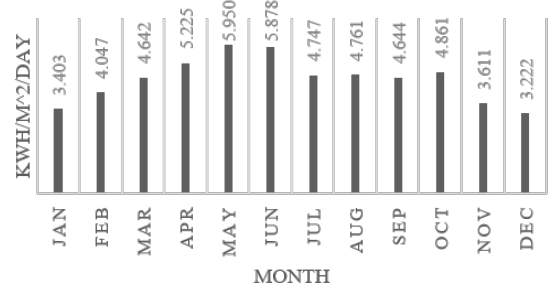
Figure 1: Mean daily global solar radiation in kWh/m 2 /day from 2008 to 2012 for Pokhara [6]
