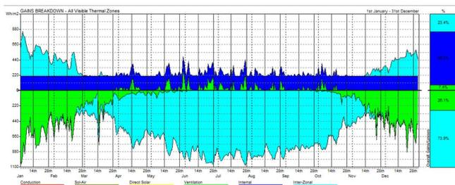
**Figure 8:** Passive Gain Breakdown when ACH= 50 in basement
