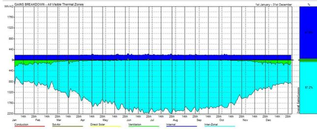
**Figure 6:** Passive Gain Breakdown existing case in basement
