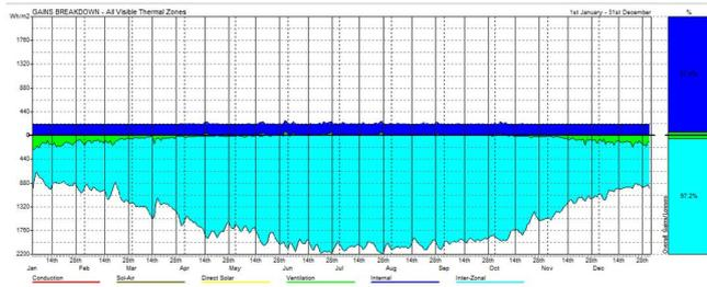
**Figure 7:** Passive Gain Breakdown when ACH= 25 in basement
