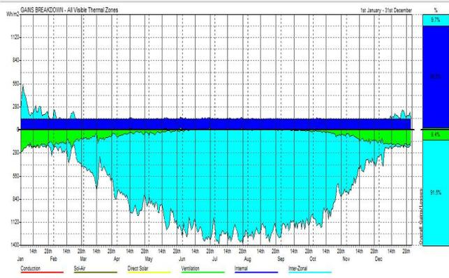
**Figure 3:** Passive Gain Breakdown in Existing Condition of Upper Floor
