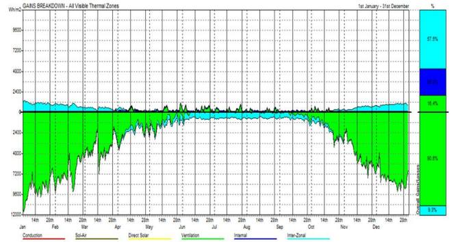
**Figure 4:** Passive Gain Breakdown When ACH=25
