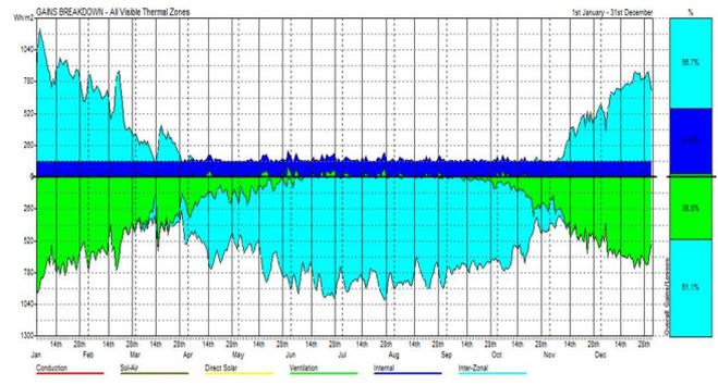
**Figure 5:** Passive Gain Breakdown When ACH=2
