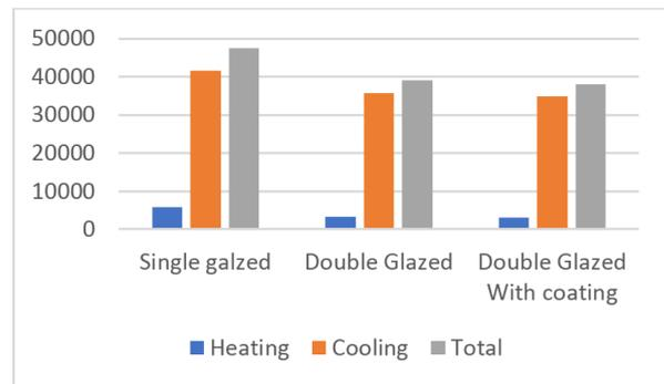
Figure 7: Energy performance of building according to glazed facade type
