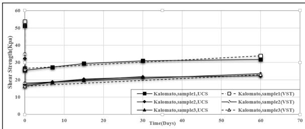
**Figure 13:** Thixotropic strength gain(Kalomato) Vs Time
