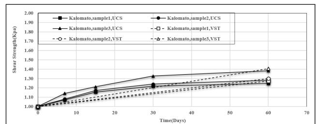
**Figure 17:** Thixotropic Strength Ratio (Kalomato) Vs Time
