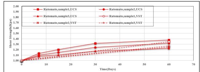
**Figure 16:** Thixotropic Strength Ratio (Ratomato) Vs Time
