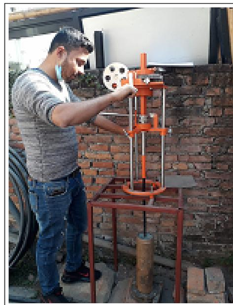
Figure 3: Vane Shear Test Setup
