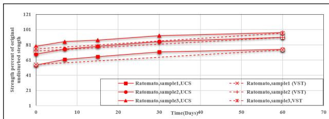
**Figure 14:** Strength Percent of original Undisturbed Strength (Ratomato) Vs Time
