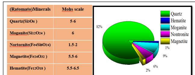
**Figure 22:** Ratomato Minerals Quantification and Hardness
