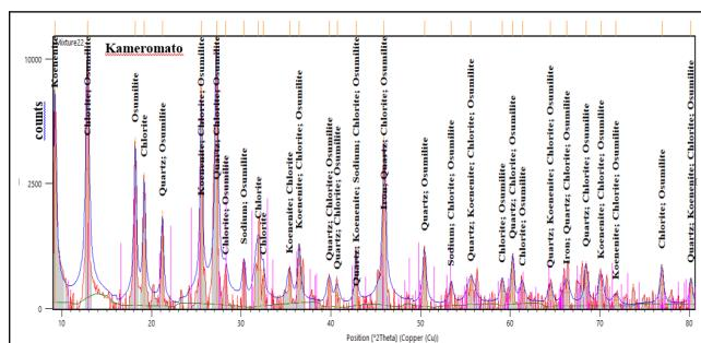
**Figure 21:** Kameromato Minerals Identification and Quantification
