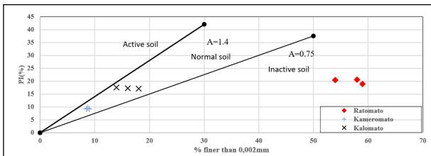
**Figure 5:** Plasticity index Vs Clay fraction
