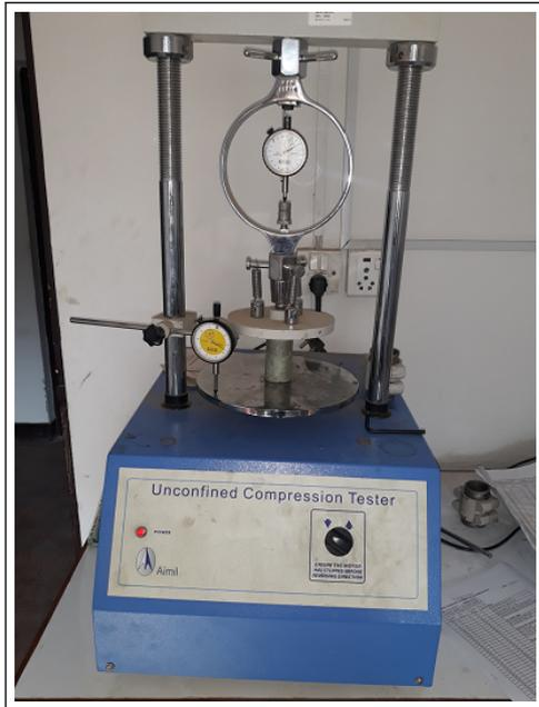
Figure 2: Unconfined Compression Test Setup
