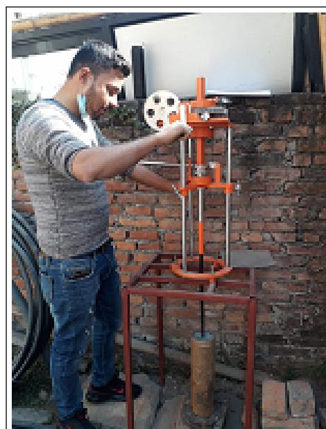
**Figure 3:** Vane Shear Test Setup
