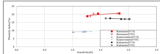
**Figure 6:** Sensitivity Vs Plasticity Index
