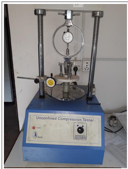
**Figure 2:** Unconfined Compression Test Setup
