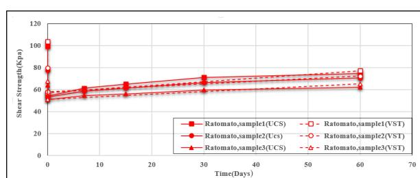
**Figure 12:** Thixotropic strength gain(Ratotmato) Vs Time
