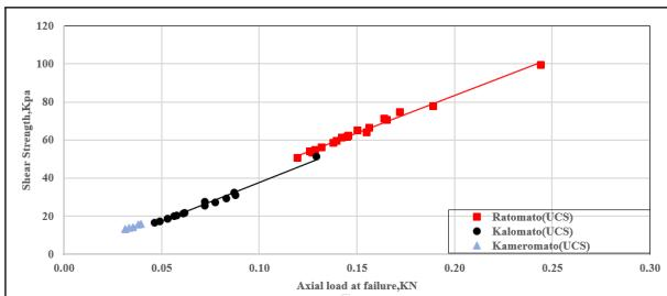
**Figure 10:** Shear Strength Vs Axial Load
