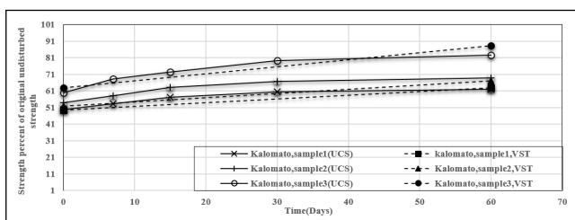
**Figure 15:** Strength Percent of original Undisturbed Strength (Kalomato) Vs Time
