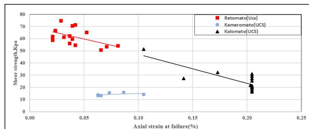
**Figure 11:** Shear Strength Vs Axial Strain
