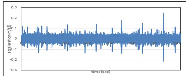
**Figure 6: Raw Acceleration Data for Jagati Bridge (Sensor Position at 1)**
