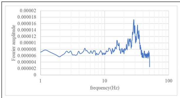
**Figure 10:** Fourier Amplitude vs Frequency (Sensor at Position 1 of Jagati Bridge)
