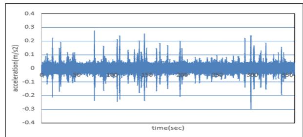
**Figure 7: Raw Acceleration Data for Jagati Bridge (Sensor Position at 2)**
