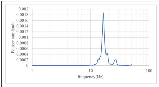
**Figure 8:** Fourier Amplitude vs Frequency (Sensor at Position 1 of Mahadev Khola Bridge)
