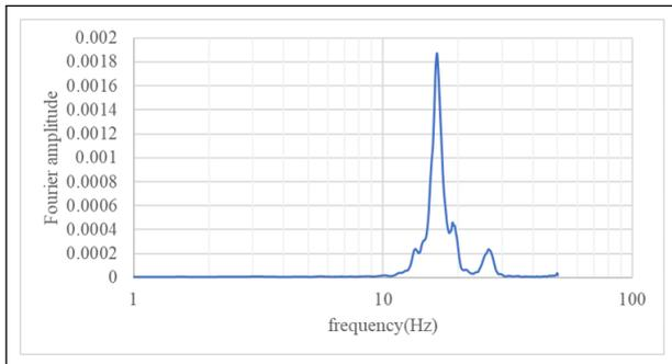
**Figure 9:** Fourier Amplitude vs Frequency (Sensor at Position 2 of Mahadev Khola Bridge)
