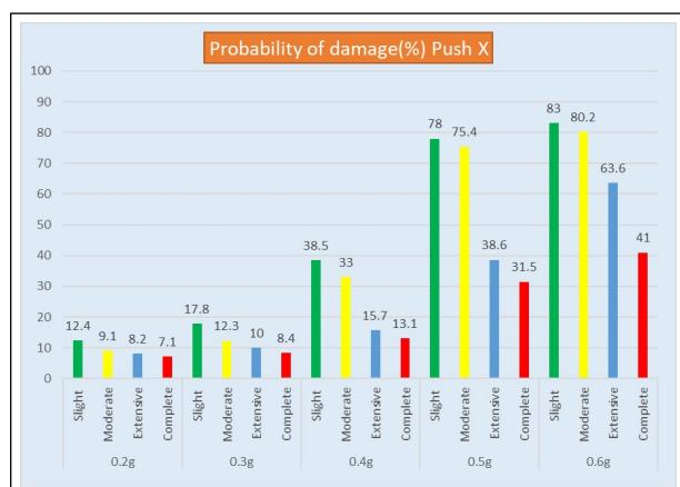
**Figure 4:** Probability of Damage (Push X)
