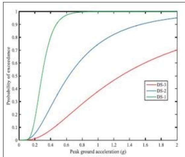
**Figure 1:** Fragility Curves with different state of Damage as a function of Peak ground acceleration(g)
