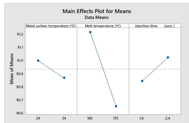
Figure 9: Main effect plot for means
