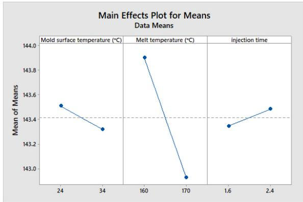
Figure 5: Main effect plot for means
