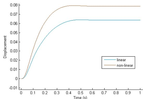
**Figure 9:** Displacement curve for semi-active linear vs non-linear model
