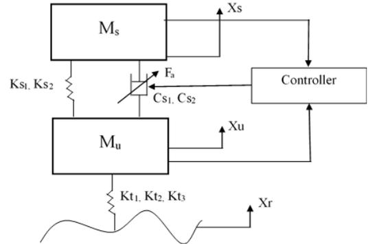
**Figure 2:** Semi active non-linear suspension system.
