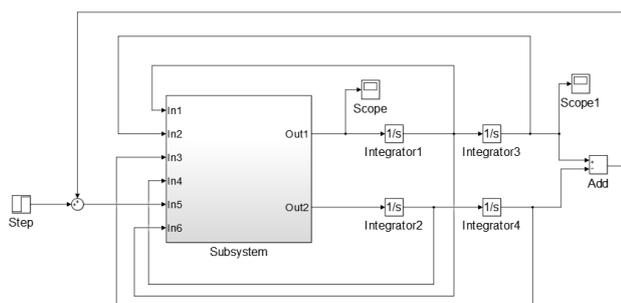
Figure 4: Semi active suspension SIMULINK model
