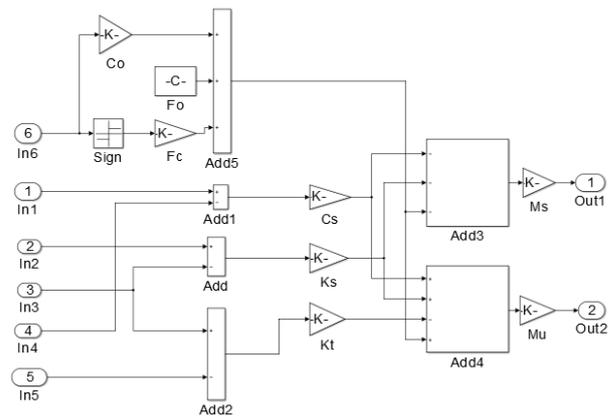
Figure 5: Subsystem for linear semi active suspension
