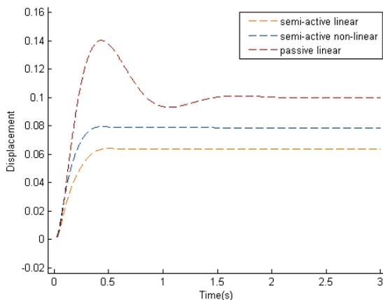
**Figure 11:** Displacement curve for passive linear vs semi-active linear vs semi-active non-linear model
