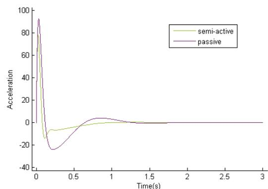
**Figure 8:** Acceleration curve for passive vs semi-active suspension
