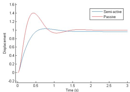
**Figure 7:** Displacement curve for passive vs semi-active suspension
