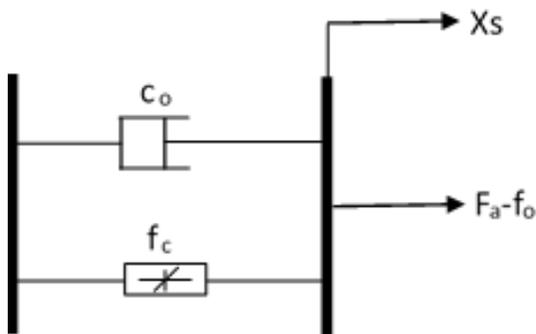
Figure 3: Bingham viscoplastic model of MR damper
