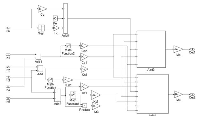
Figure 6: Subsystem for non-linear semi active suspension
