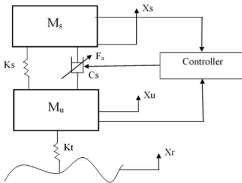
**Figure 1:** Semi active linear suspension system.
