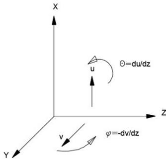
**Figure 8:** Relation between angular and transverse displacements
