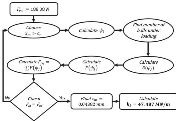
**Figure 3:** Stiffness of bearings
