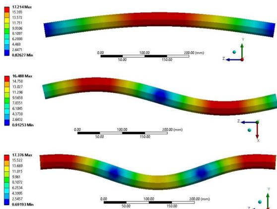
**Figure 6:** First three mode shapes from ANSYS
