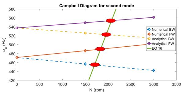
Figure 10: Variation of second mode natural frequency with rotational speed
