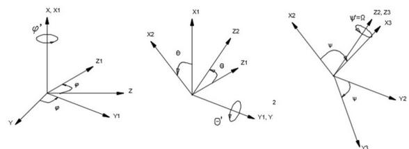
**Figure 7:** Rotation angles achieved by disk and shaft
