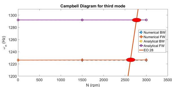
Figure 11: Variation of third mode natural frequency with rotational speed
