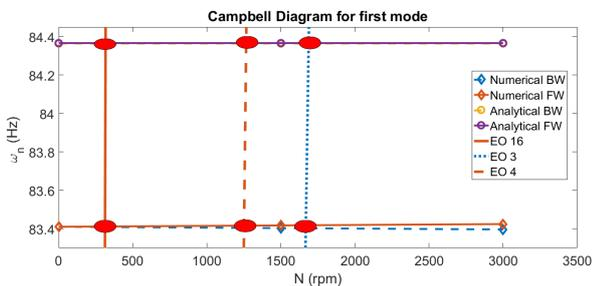
Figure 9: Variation of first mode natural frequency with rotational speed
