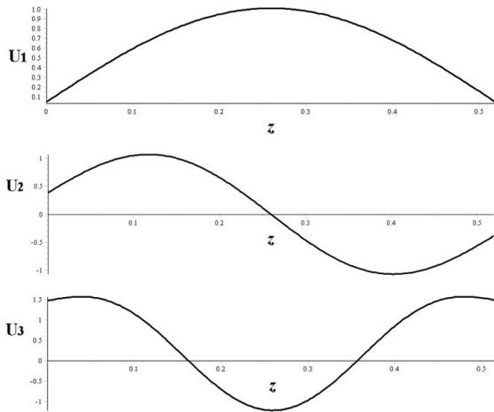
**Figure 5:** First three mode shapes
