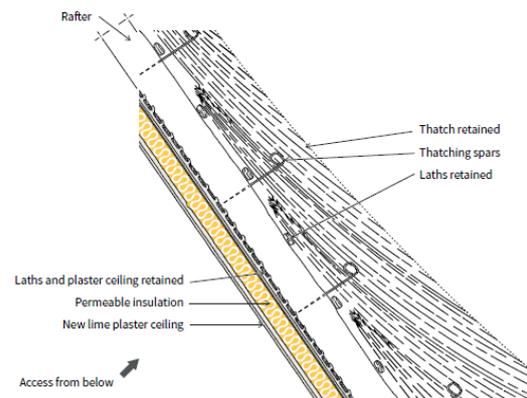
Figure 14: Warm roof – sloping ceiling (White, 2012)
