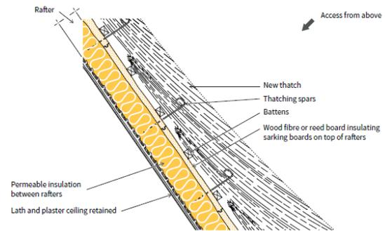
Figure 13: Warm roof – sloping ceiling (White, 2012)
