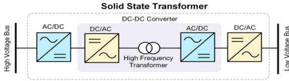
Figure 1: Block Diagram Representation of SST
