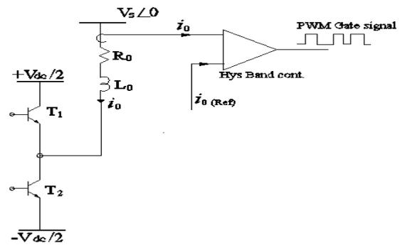
**Figure 5:** Schematic Diagram of HBCC
