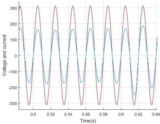
Figure 11: Input Voltage and Current Waveform
