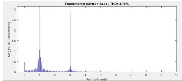
Figure 15: Harmonic Content in Output Voltage
