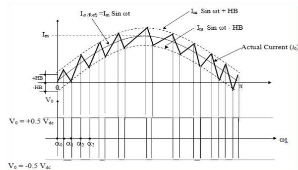
**Figure 6:** Switching Instants and Waveforms of HBCC PWM Inverter
