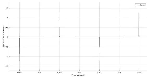
**Figure 4:** Spikes in Input Current Drawn by Non-Linear Load
