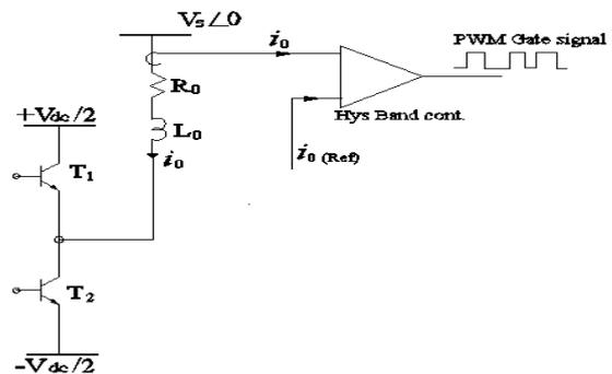
**Figure 5:** Schematic Diagram of HBCC
