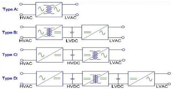
Figure 2: Different Topologies of SST
