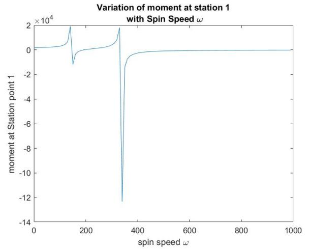
Figure 4.5: Variation of moment at station 1 with spin speed
