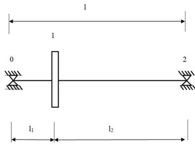
Figure 2.3: Schematic model for rotor model
