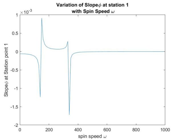
Figure 4.6: Variation of slope at station 1 with spin speed
