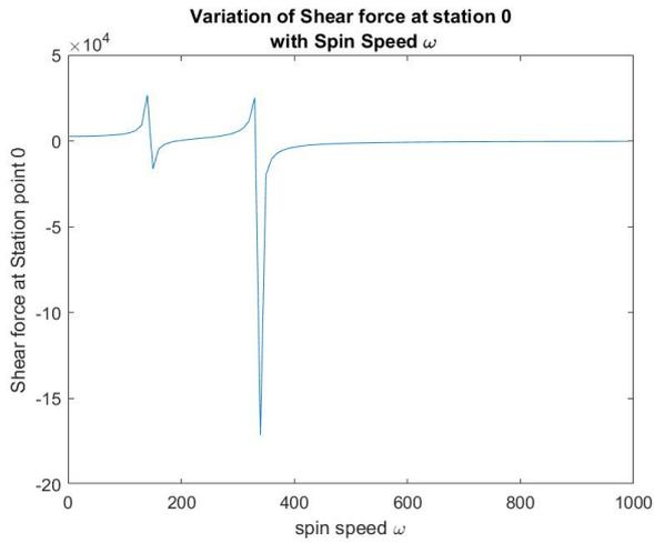
Figure 4.2: Variation of Shear force at station 0 with spin speed
