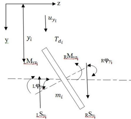
Figure 2.5: Free body diagram of disk element
