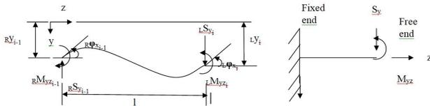
Figure 2.4: Free body diagram of general shaft element
