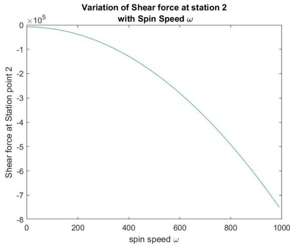
**Figure 4.8:** Variation of Shear force at station 2 with spin speed
