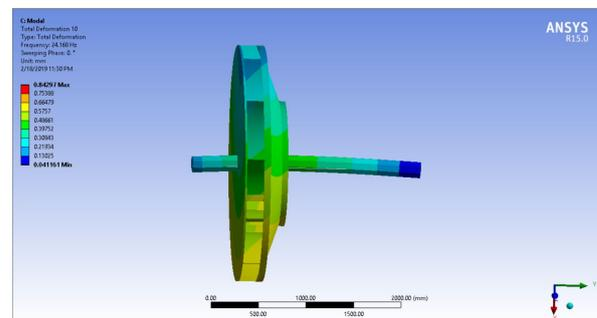
**Figure 4.10:** Displacement at 144.2495 rad/s
