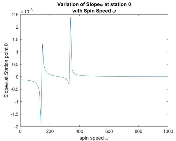
**Figure 4.1:** Variation of slope at station 0 with spin speed
