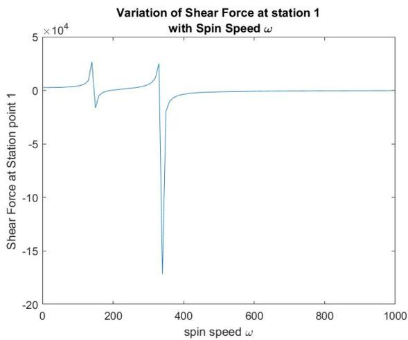
Figure 4.4: Variation of Shear force at station 1 with spin speed
