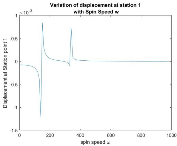
Figure 4.3: Variation of displacement at station 1 with spin speed
