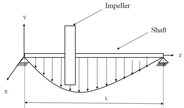
**Figure 2.2:** Schematic diagram of rotor system
