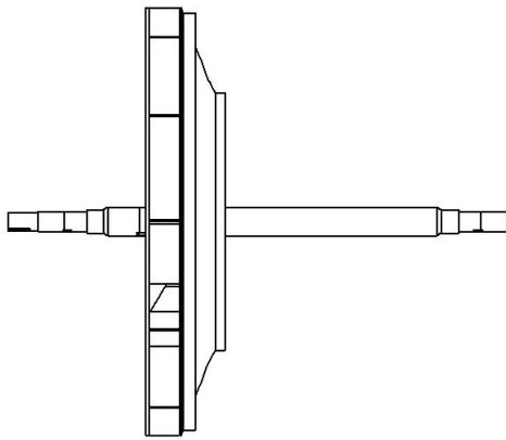
**Figure 2.1:** CAD model of offset rotor shaft of centrifugal fan
