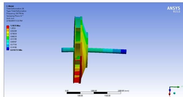
**Figure 4.11:** Displacement at 335.0 rad/s
