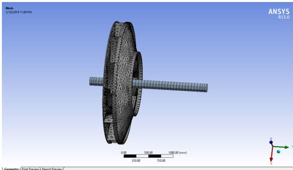
**Figure 3.3:** Mesh development for rotor dynamic shaft
