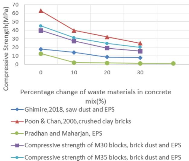
**Figure 9:** Variation of compressive strength with percentage change of waste material in constituent concrete
