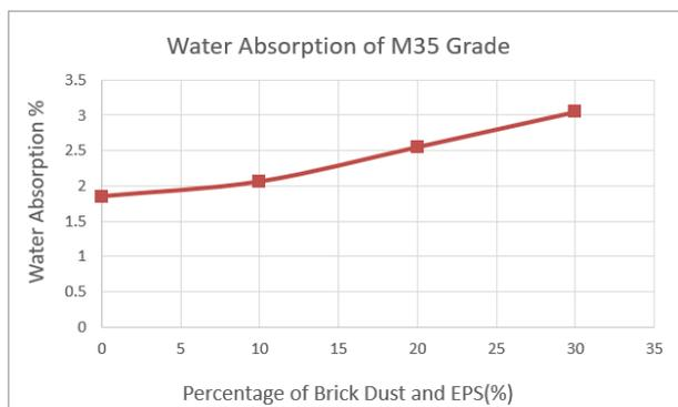
**Figure 6:** variation of Water Absorption of M35 Grade Concrete containing different percentage of Brick Dust and EPS
