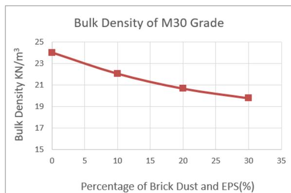
**Figure 7:** variation of Bulk Density of M30 Grade Concrete containing different percentage of Brick Dust and EPS
