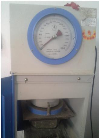
**Figure 2:** Paving blocks under compressive loading
