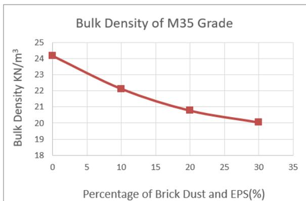
**Figure 8:** variation of Bulk Density of M35 Grade Concrete containing different percentage of Brick Dust and EPS
