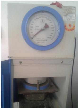
**Figure 2:** Paving blocks under compressive loading
