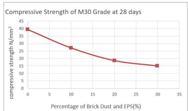
**Figure 3:** variation of Compressive Strength of M30 Grade Concrete containing different percentage of Brick Dust and EPS
