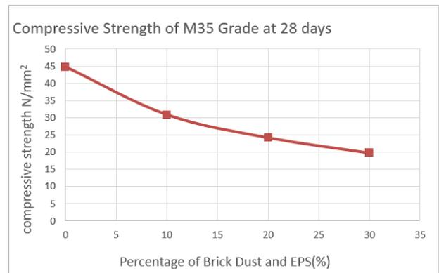
Figure 4: variation of Compressive Strength of M35 Grade Concrete containing different percentage of Brick Dust and EPS
