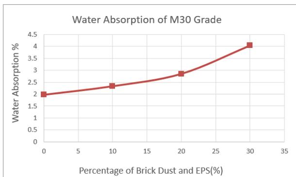
**Figure 5:** variation of Water Absorption of M30 Grade Concrete containing different percentage of Brick Dust and EPS
