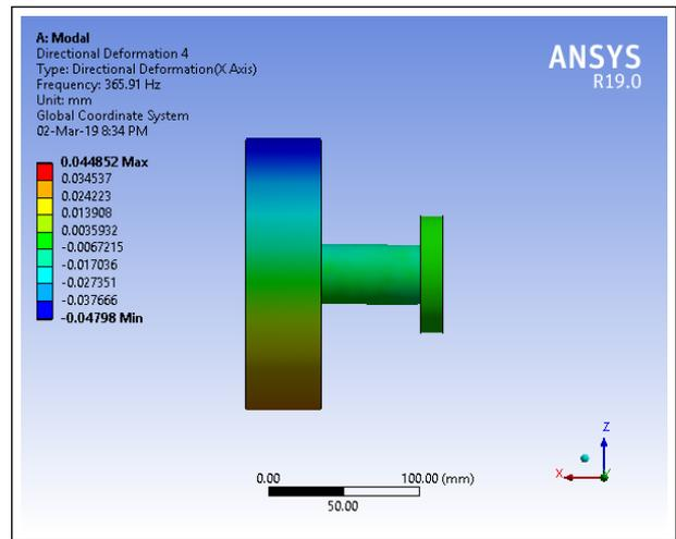
Figure 5: Directional deformation and stress distribution for Third mode of vibration
