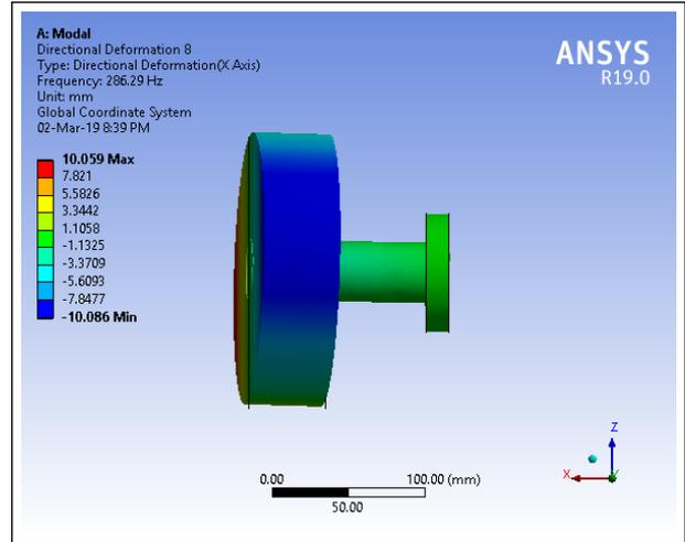
Figure 4: Directional deformation and stress distribution for Second mode of vibration
