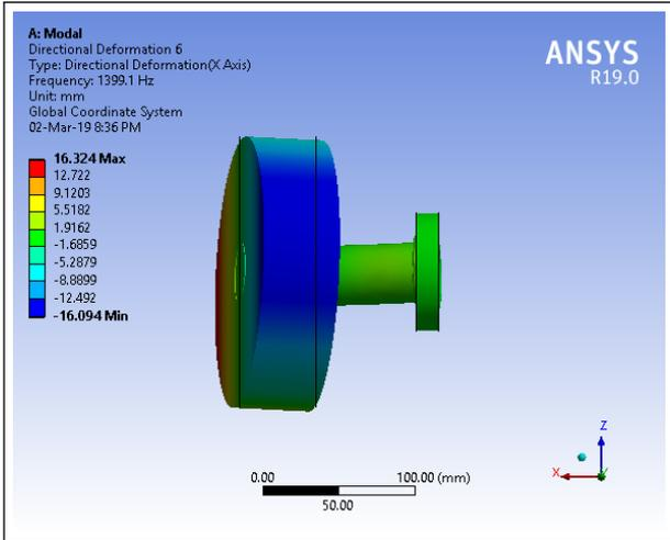
Figure 7: Directional deformation and stress distribution for Fifth mode of vibration
