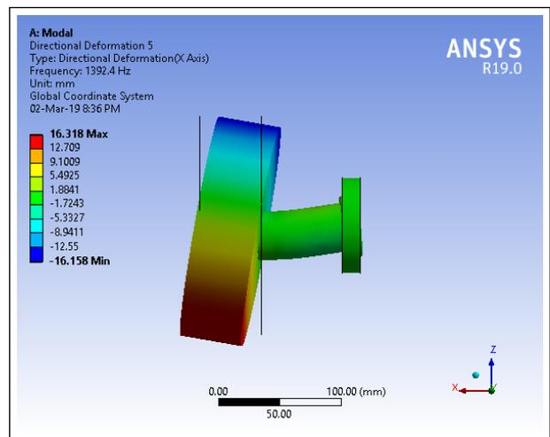
Figure 6: Directional deformation and stress distribution for Fourth mode of vibration
