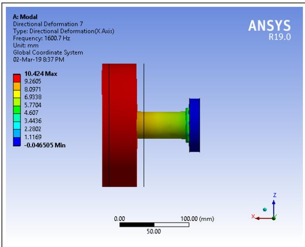
Figure 8: Directional deformation and stress distribution for Sixth mode of vibration
