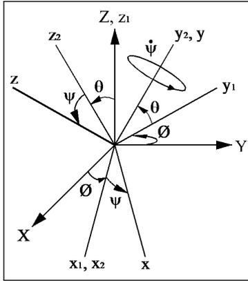
Figure 1: rotational matrix for 312 euler angles
