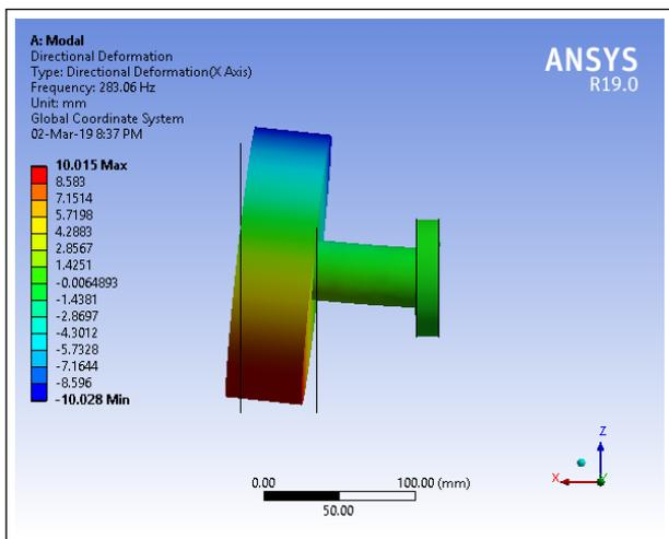
Figure 3: Directional deformation and stress distribution for First mode of vibration
