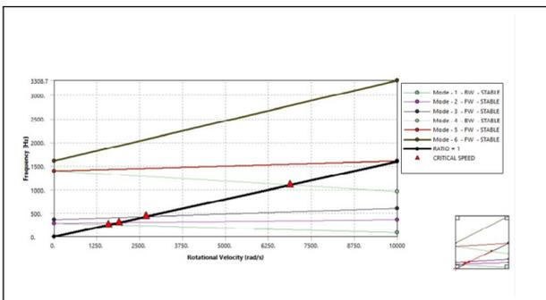
Figure 9: Campbell diagram from ANSYS simulation
