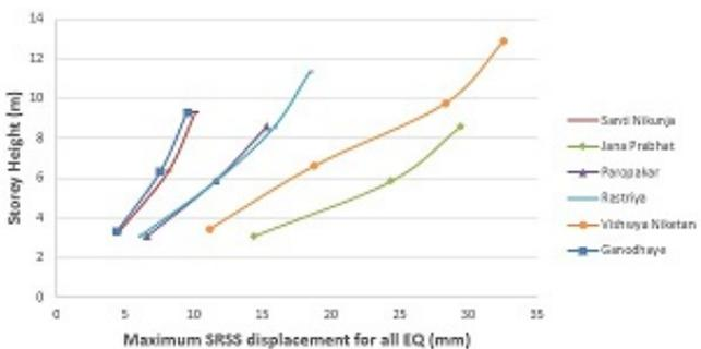
**Figure 21:** Comparative analysis of L-shaped with rectangular for max. SRSS displacement response
