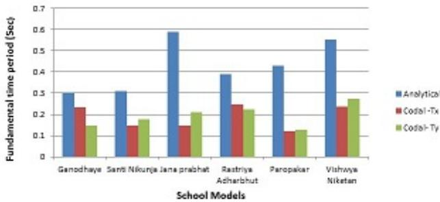
**Figure 20:** Variation of the analytical time period with the code along both directions
