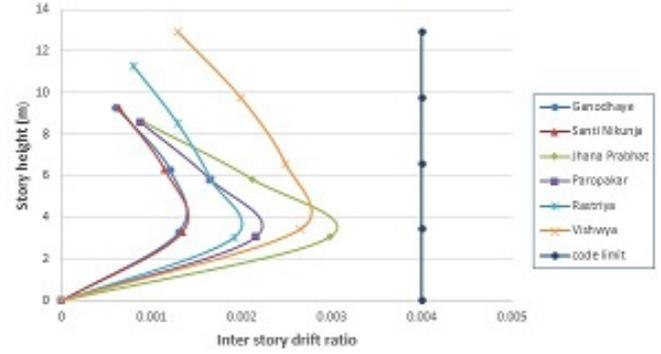
**Figure 22:** Comparative analysis of L-shaped with rectangular for max. SRSS inter story drift response
