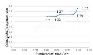
Figure 16: Variation of the max. by global response with time for inter story drift
