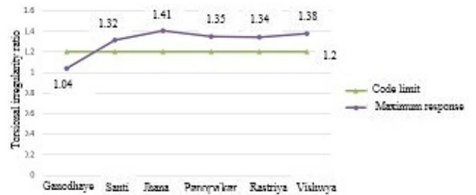
**Figure 23:** Comparative analysis of L-shaped with rectangular for max. SRSS torsion coefficient response
