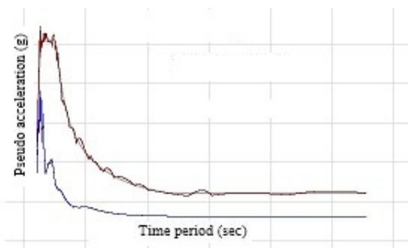
Figure 13: Response spectrum of original, matched and target spectrum for Darfield EQ
