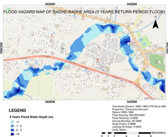
**Figure 12:** Flood hazard map (Radhe-Radhe area) of 5 years Return Period Flood
