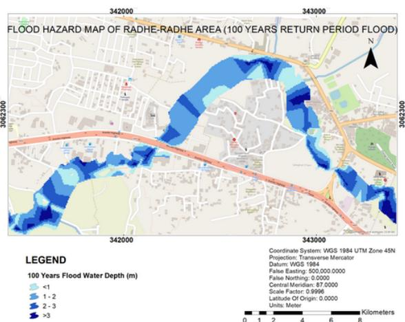
**Figure 16:** Flood hazard map (Radhe-Radhe area) of 100 years Return Period Flood
