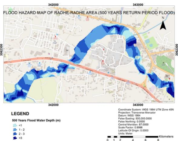
**Figure 17:** Flood hazard map (Radhe-Radhe area) of 500 years Return Period Flood
