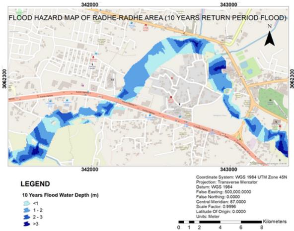
**Figure 13:** Flood hazard map (Radhe-Radhe area) of 10 years Return Period Flood
