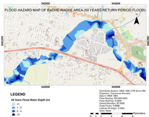
**Figure 15:** Flood hazard map (Radhe-Radhe area) of 50 years Return Period Flood
