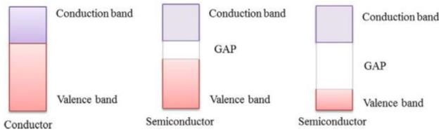
**Figure 1:** Band of valence, band gap (GAP) and the conduction band: insulator, conductor
