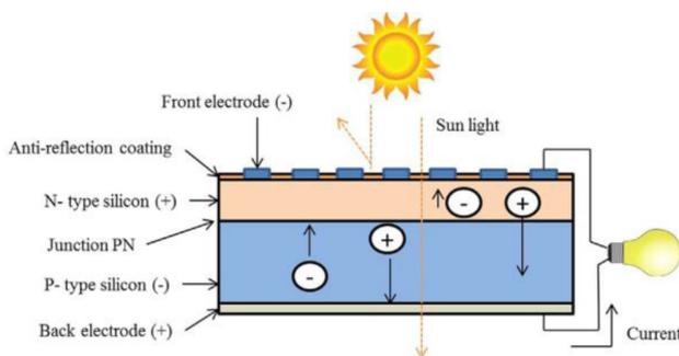
**Figure 2:** Photovoltaic Cell
