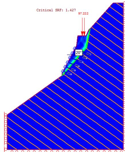
**Figure 7:** Result: Anchors oriented horizontally
