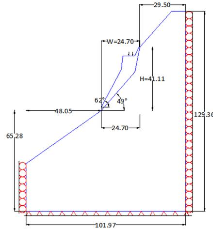
Figure 2: Slope model
