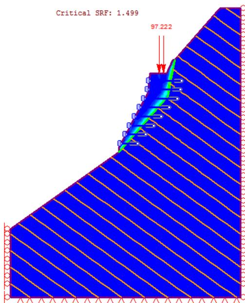
**Figure 6:** Result: Anchors oriented at 20 degree
