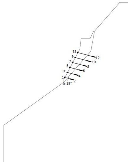
Figure 3: Slope model with anchors
