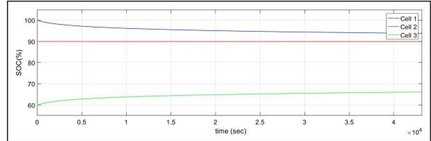
**Figure 14:** SoC of Cells in Active Balancing for 3.3V
