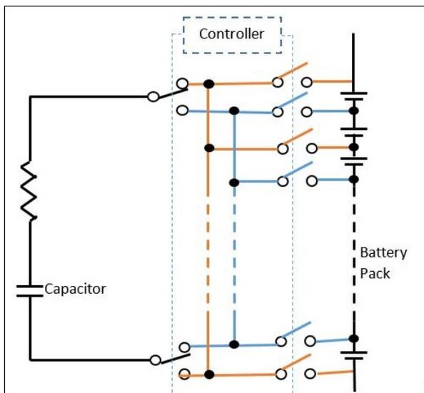
**Figure 4:** Single Switched Capacitor topology of Active Cell Balancing
