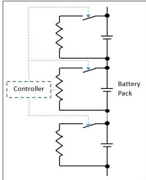
Figure 2: Switched Shunt Resistor topology of Passive Cell balancing
