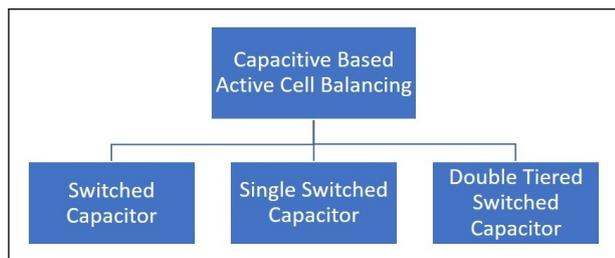
**Figure 3:** Active Cell Balancing Topologies using Capacitor
