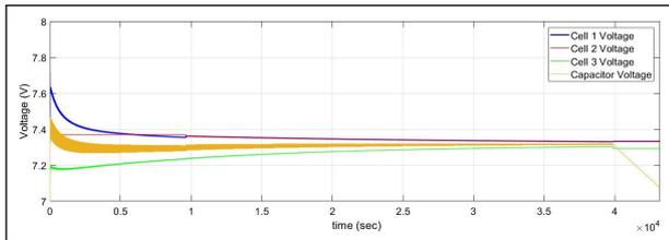
**Figure 19:** Voltages in Active Balancing for 7.1V
