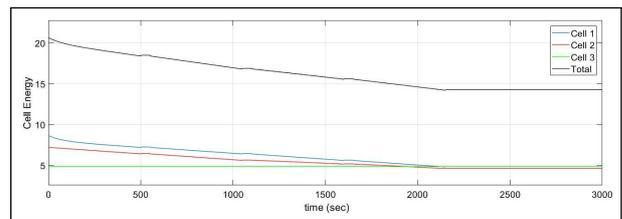
**Figure 9: Energy Content of Cells in Passive balancing for 3.3V**
