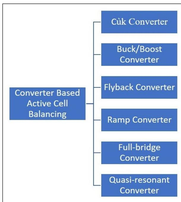
**Figure 5:** Active Cell Balancing Topologies using Converters
