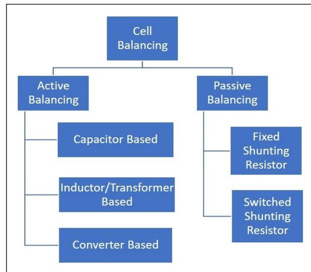
Figure 1: Active and Passive Cell Balancing Topologies
