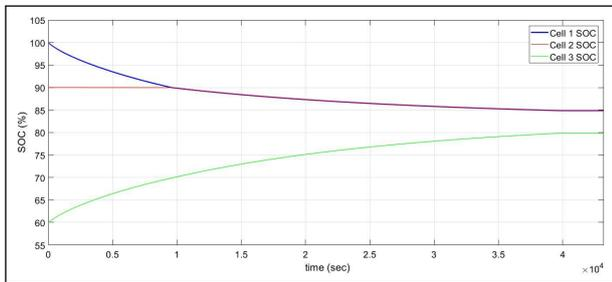
**Figure 18:** SoC of Cells in Active Balancing for 7.1V
