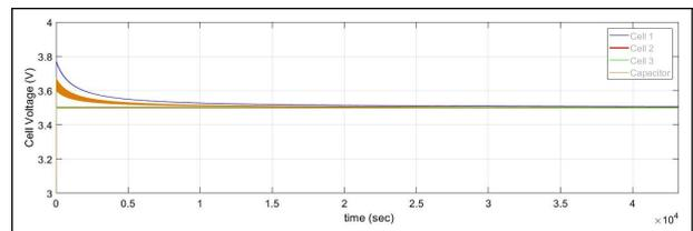
**Figure 15:** Voltages in Active Balancing for 3.3V
