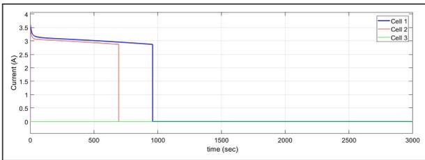
**Figure 12:** Resistor Current in Passive Balancing 7.1V
