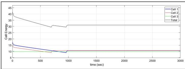
**Figure 13:** Energy Content of Cells in Passive balancing for 7.1V
