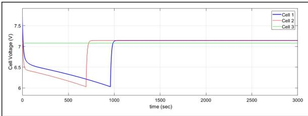
**Figure 11:** Cell Voltage in Passive Balancing for 7.1V
