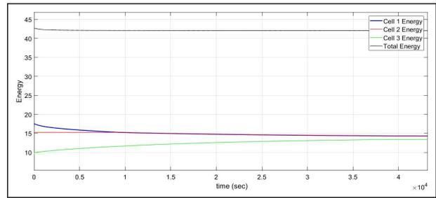
**Figure 21:** Energy Content of Cells in Active Balancing for 7.1V
