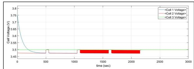
Figure 7: Cell Voltage in Passive Balancing for 3.3V
