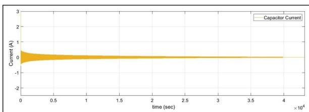
**Figure 20:** Capacitor Current in Active Balancing for 7.1V
