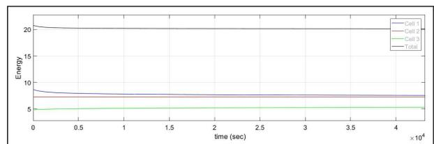
**Figure 17:** Energy Content of Cells in Active Balancing for 3.3V
