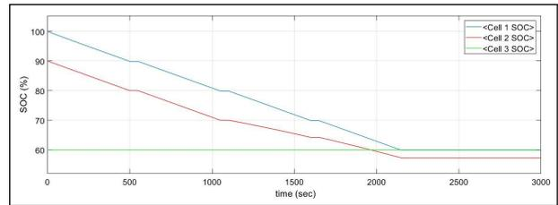
**Figure 6: SoC of Cells in Passive Balancing for 3.3V**
