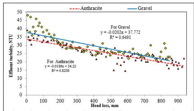
**Figure 5:** Effluent turbidity vs. Head loss
