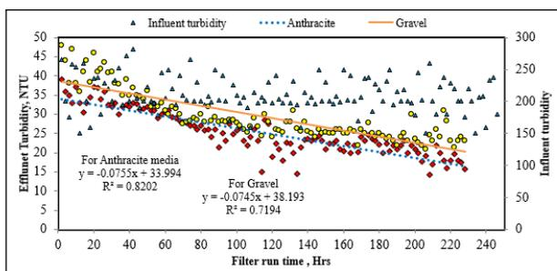
**Figure 4:** Turbidity vs Filter run time at 1.00m/h
