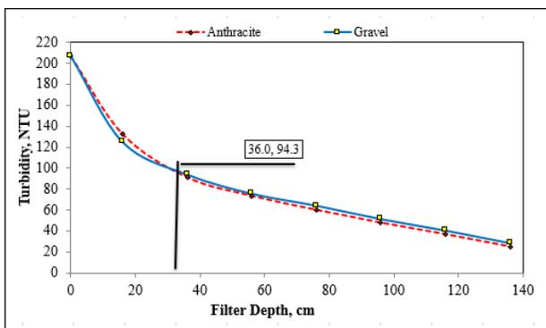
Figure 7: Turbidity Removal profile along filter depth at 1 m/h
