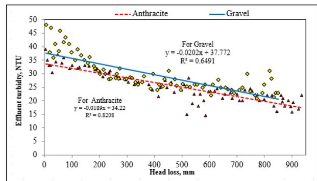
Figure 5: Effluent turbidity vs. Head loss
