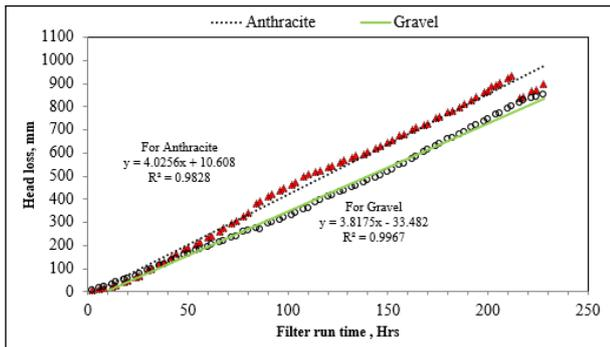
Figure 6: Head loss vs. filter run time at 1.00m/h
