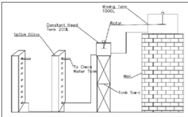
Figure 1: Schematic diagram of filter model setup
