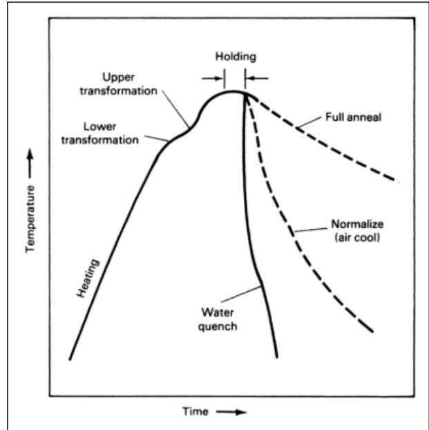
**Figure 9:** Heat Treatment(Hardening) Process
