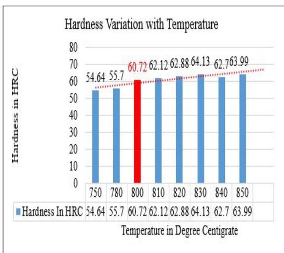
Figure 12: Hardness Variation with Heating Temperature
