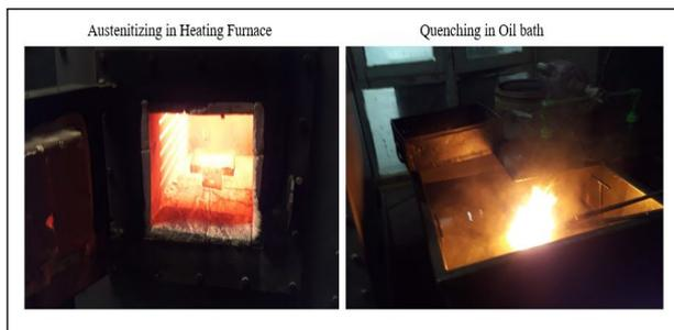
Figure 11: Heating and Quenching of Samples
