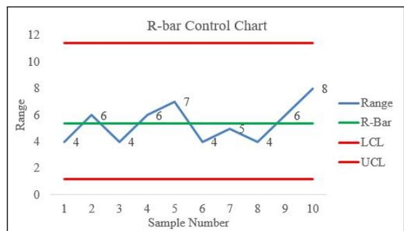
Figure 6: R-bar Control Chart before Standardization
