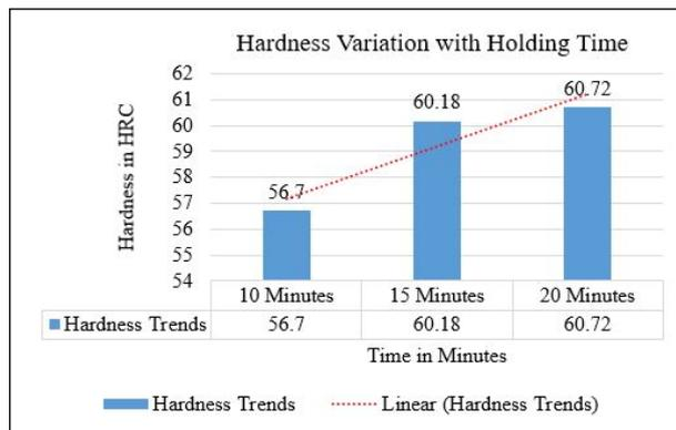
Figure 13: Hardness Variation with Holding Time at Constant Temperature
