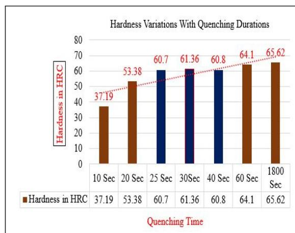
Figure 14: Hardness Variation with Quenching Time (Oil Bath at Room Temperature)
