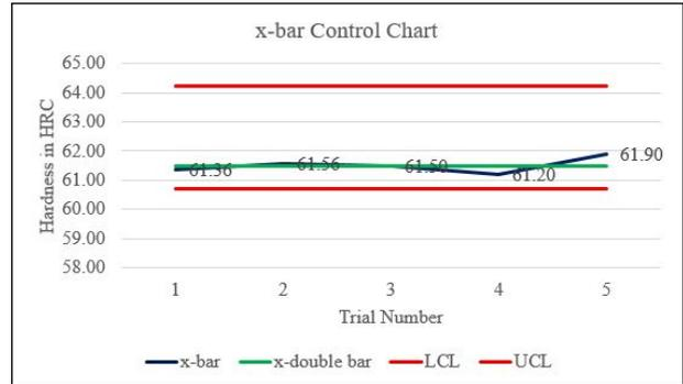
**Figure 15:** X-bar Control Chart after Standardization
