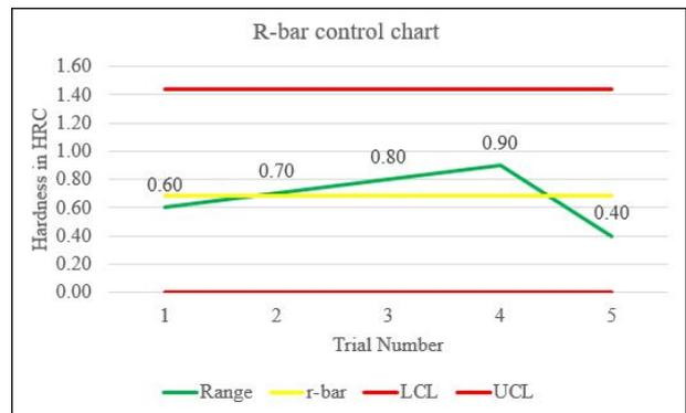
**Figure 16:** R-bar Control Chart after Standardization
