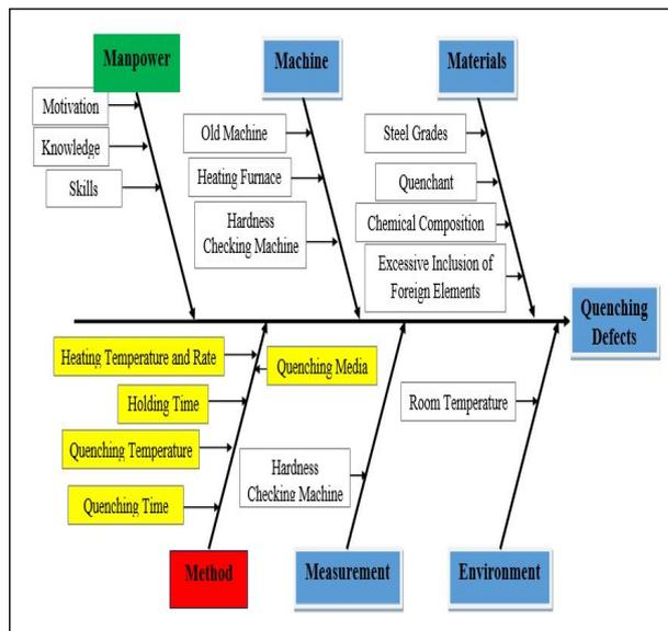
Figure 7: Ishikawa Diagram for Quenching Defects
