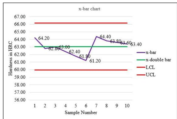
Figure 5: X-bar Control Chart before Standardization
