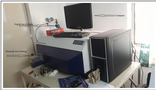
**Figure 8:** Digital Metal Analyzer(Spectrometer)
