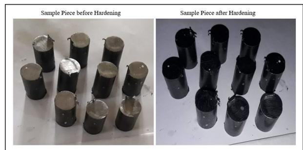
**Figure 10:** Samples of 100Cr6 for Experiment
