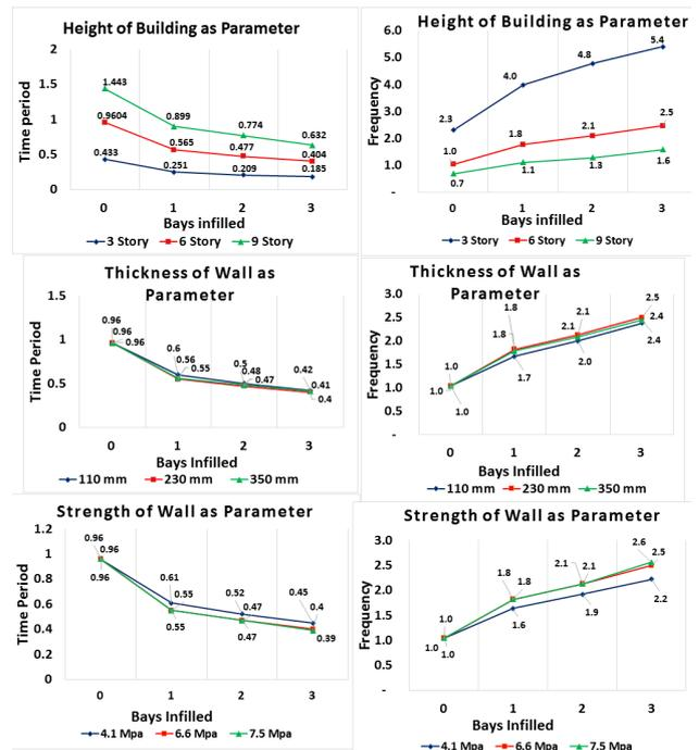
Figure 12: First mode time periods and frequencies for different parameters with different infill configurations
