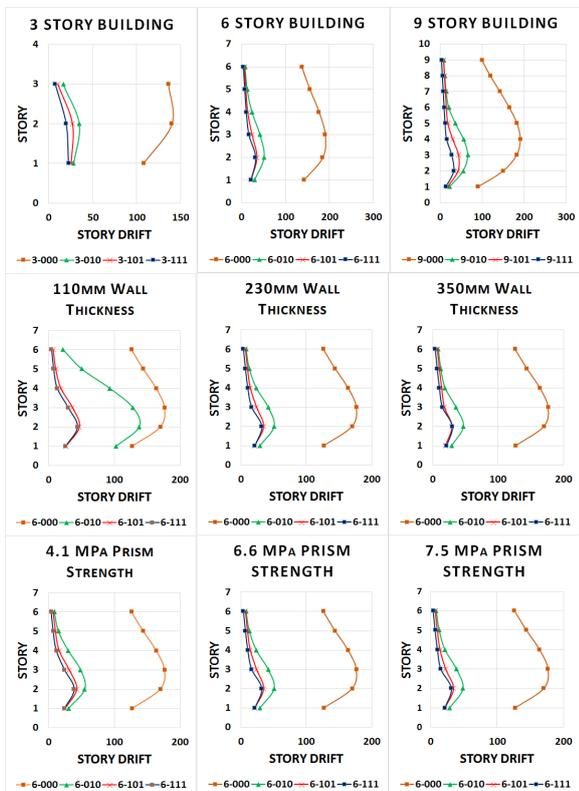
Figure 11: Inter story drifts compared to different parameters with different infill configurations
