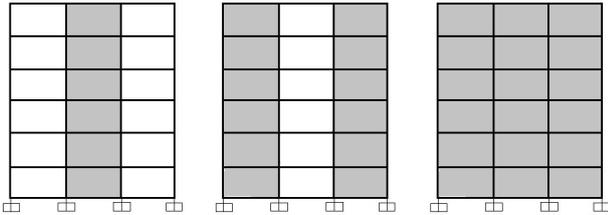
Figure 5: Six story building with 0-1-0, 1-0-1 and 1-1-1 infill wall configurations
