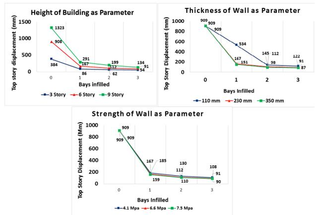
Figure 9: Top story displacement vs number of bays infilled for different parameters
