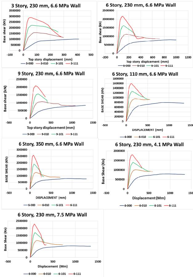
Figure 7: Pushover curves of different buildings for parametric analysis
