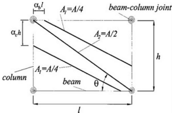
**Figure 2:** Equivalent three diagonal strut model for masonry infilled frames.
