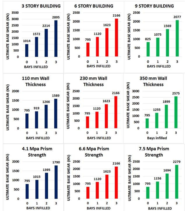
Figure 8: Ultimate strength for different parameters compared to the number of bays infilled
