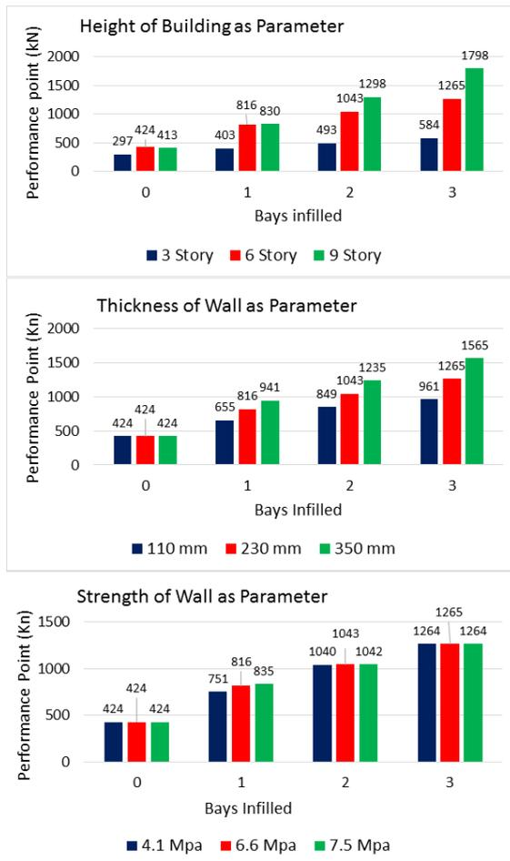
Figure 13: Performance points for buildings with different parameters
