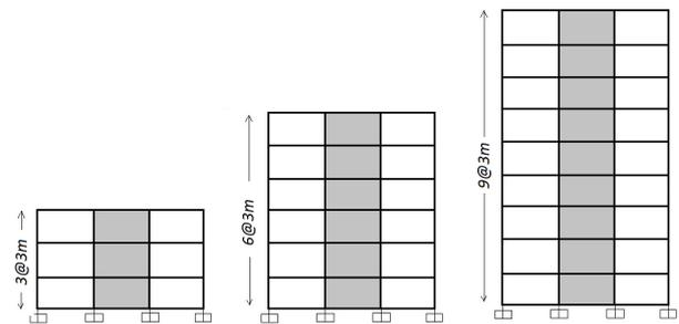
**Figure 3:** Low-rise, mid-rise, and high-rise building with mid bay infilled (0-1-0)
