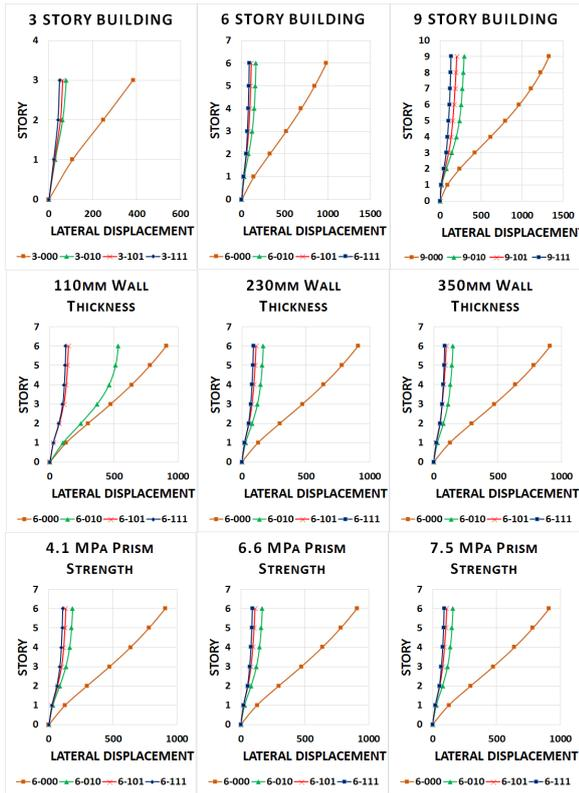
Figure 10: Total displacement at each story for different parameters with different infill configurations
