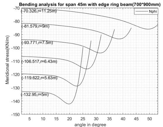
Figure 5: meridional stresses for the spherical shells with span 45 m supported on edge ring beam
