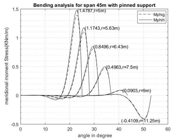
Figure 4: Meridional moment for pinned support spherical shells with fixed span 45m and different rises
