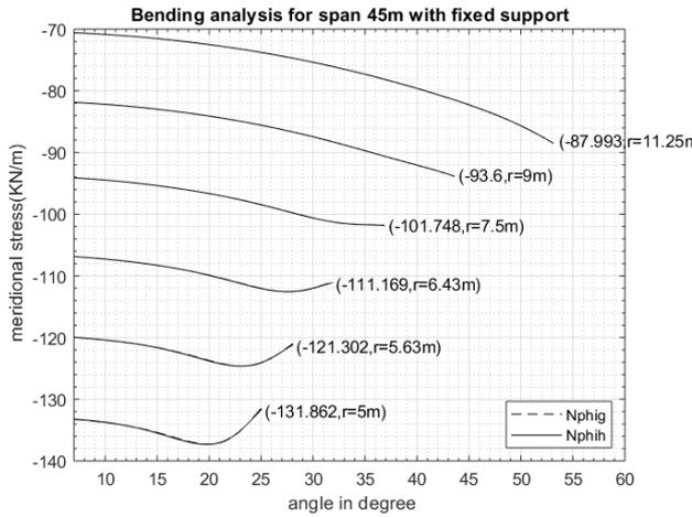
Figure 1: meridional Stresses for clamped support spherical shells with fixed span 45m and different rises
