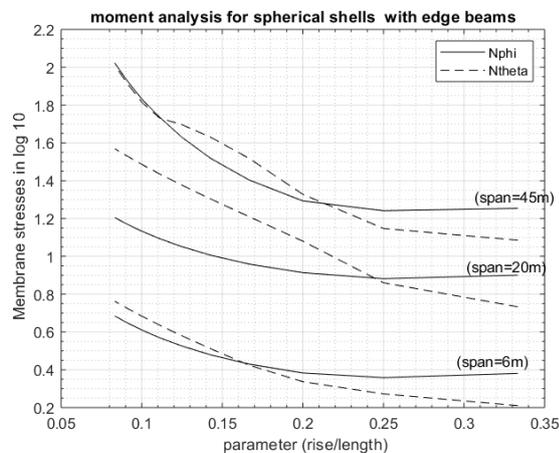
Figure 13: membrane stresses for spherical shells with different rise/span ratio for edge beam with gradually varying thickness
