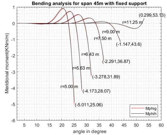
Figure 3: Meridional moment for clamped support with fixed span 45 m and different rises
