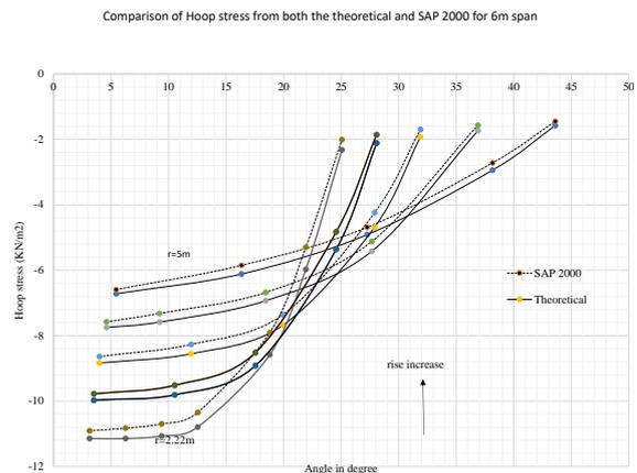
**Figure 9:** hoop stress of 6 m span shell from SAP 2000 compared with theroretical method
