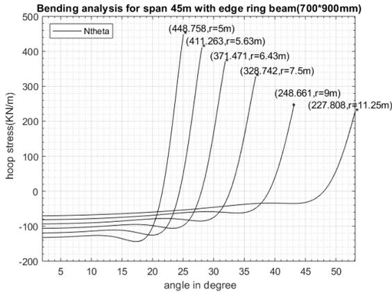
**Figure 6:** meridional stresses for the spherical shells with span 45 m supported on edge ring beam
