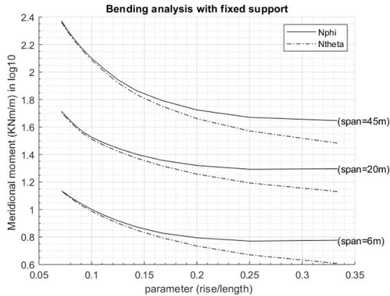
Figure 11: membrane stresses for fixed span spherical shells with different rise/span ratio for fixed support
