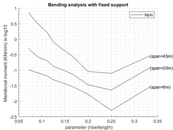
Figure 12: Moment stresses for fixed span spherical shells with different rise/span ratio for pinned support
