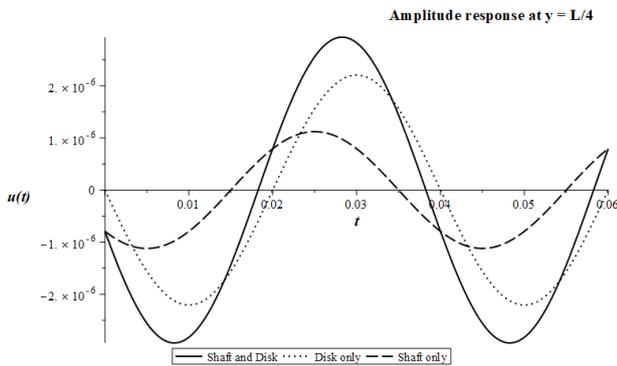
Figure 5: Transverse displacement at  $y = L/4$  in horizontal direction for  $\Omega = 1500 RPM$
