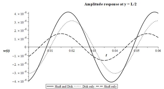
Figure 8: Transverse displacement at  $y = L/2$  in vertical direction for  $\Omega = 1500 RPM$
