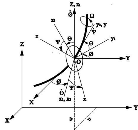
Figure 2: Disk rotating on flexible shafts with reference frames [5]
