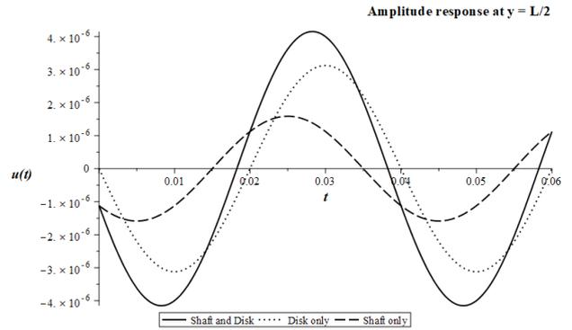
Figure 7: Transverse displacement at  $y = L/2$  in horizontal direction for  $\Omega = 1500 RPM$
