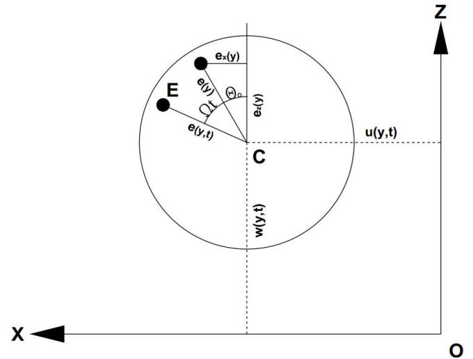
Figure 4: Mass unbalance in shaft
