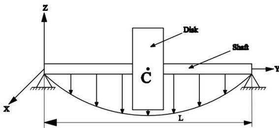
Figure 1: Shaft and Disk assembly with supports [4]
