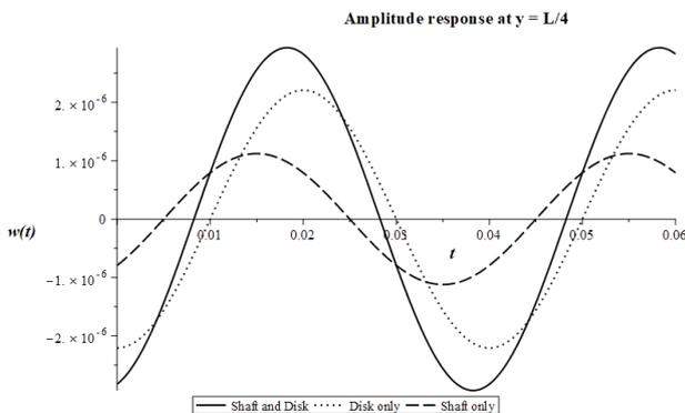
Figure 6: Transverse displacement at  $y = L/4$  in vertical direction for  $\Omega = 1500 RPM$
