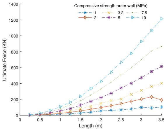
**Figure 6:** Ultimate force versus length for different compressive strength
