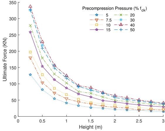
**Figure 5:** Ultimate force versus height for different precompression ratios
