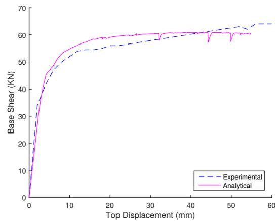
**Figure 4:** Pushover curve of wall SNK 7.5: Analytical and Experimental
