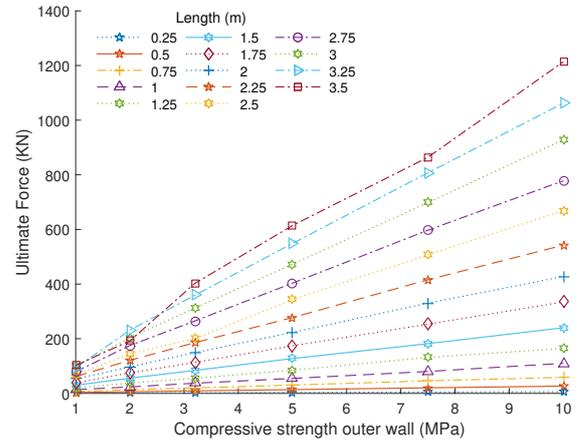
**Figure 8:** Ultimate force versus compressive strength for different lengths
