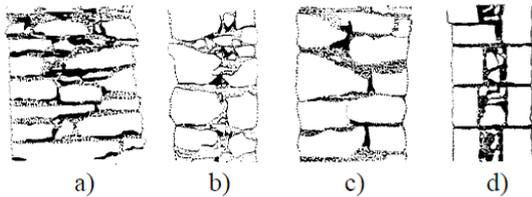
**Figure 1:** Stone Masonry classification by cross section: a) single leaf or solid, b) two leaves without connection, c) two leaves with connection, d) three leaves (Figure Courtesy : [18])
