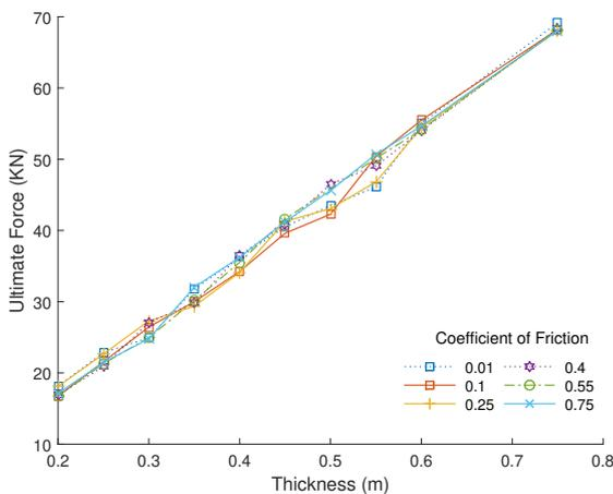
**Figure 7:** Ultimate force versus thickness for different coefficient of friction
