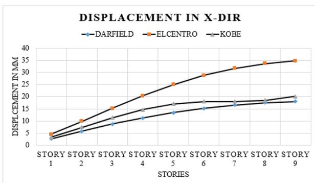
**Figure 2:** Displacements in x-direction due to various earthquake force in G + 8 RCC
