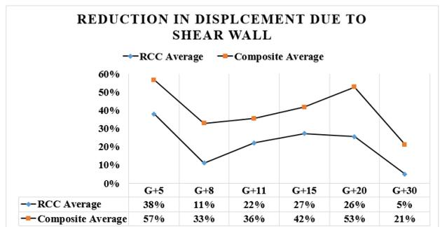
Figure 23: Reduction in displacement due to shear wall
