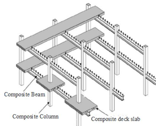
Figure 1: Composite Structure elements
