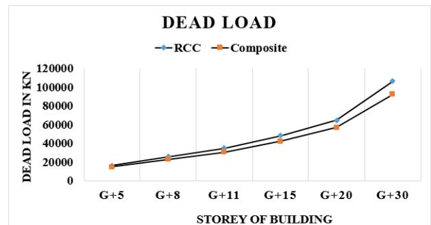
Figure 7: Dead load comparison between RCC and composite
