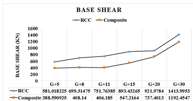
Figure 9: Base Shear comparison between RCC and composite
