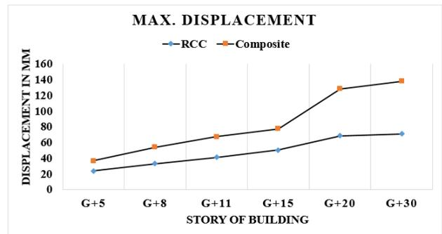
Figure 11: Max Displacements of buildings
