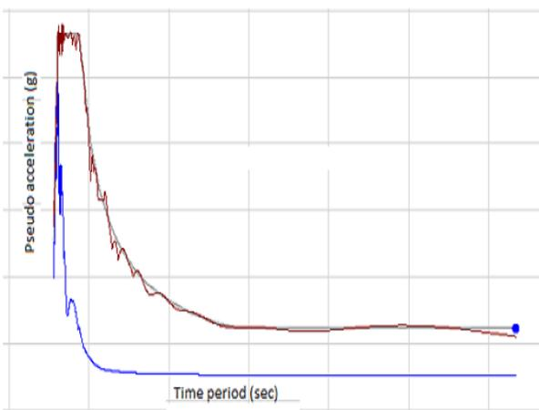
**Figure 3:** Response spectrum of original, matched and target spectrum for Imperial earthquake
