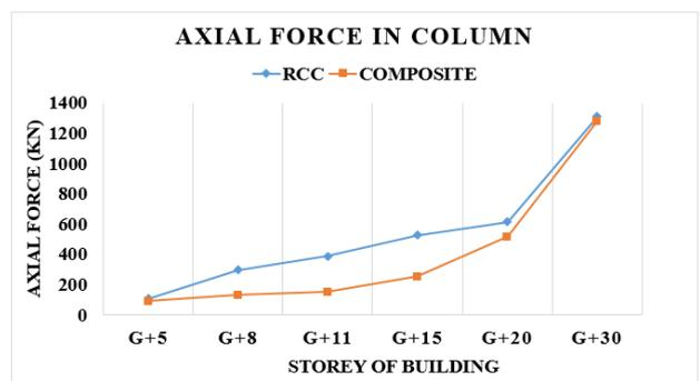
Figure 17: Axial force in columns
