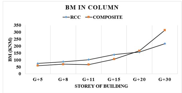
Figure 21: Bending Moment in columns
