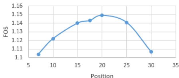
Figure 8: Plot of FOS and Position (from Top of slope) for phi 41 degrees
