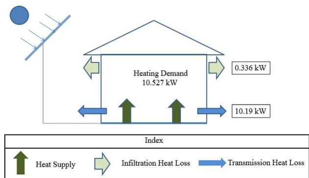
**Figure 6:** Overall Heating Load
