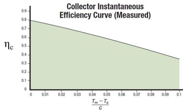
**Figure 4: Typical Collector Efficiency Curve**
