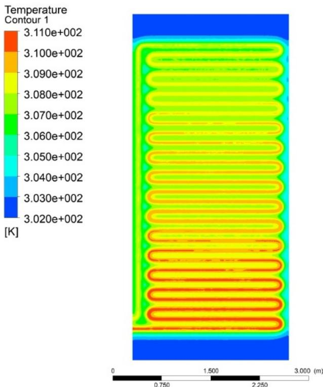
Figure 7: Analysis of Serpentine Loop
