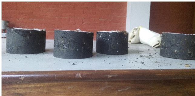
Figure 8: Samples with cement and stone dust as filler; darker black colour
