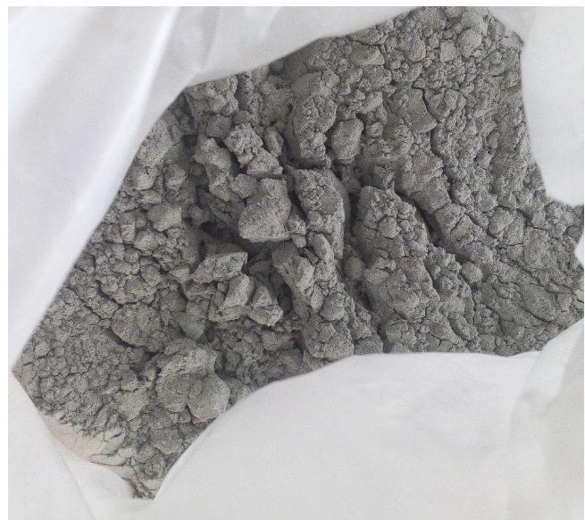
Figure 7: Fly ash with its natural greyish color
