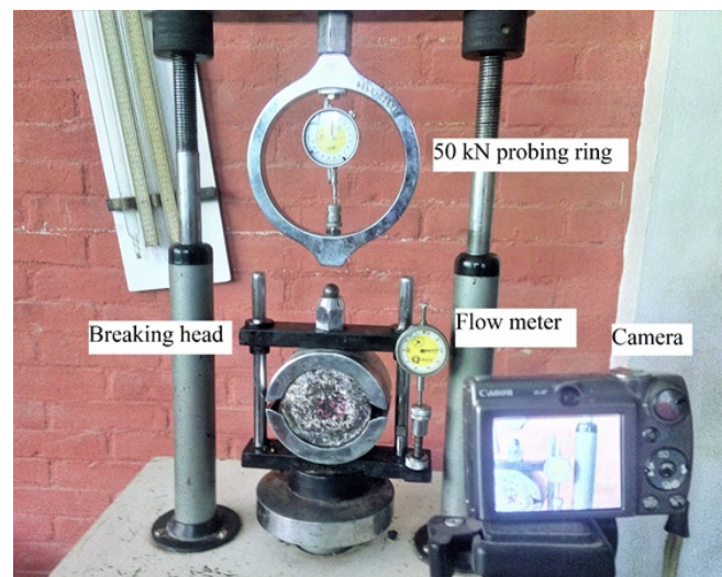
Figure 10: Marshall stability test setup in Kantipur Engineering College, Dhapakhel
