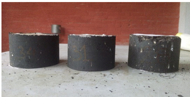
Figure 9: Samples with fly ash as filler; greyish colour in the surface
