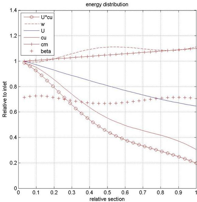
Figure 6: Energy distribution along streamline
