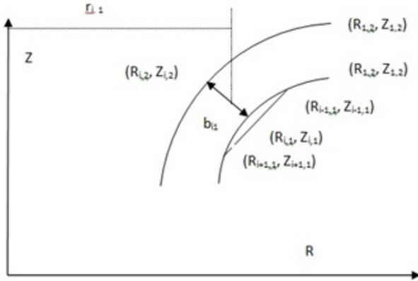
**Figure 3:** finding a new point on streamline
