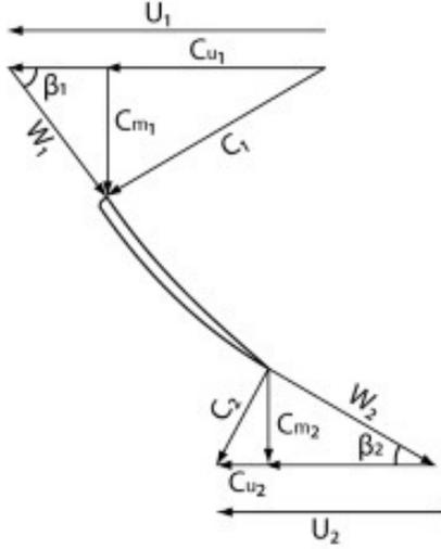
**Figure 2:** velocity diagram
