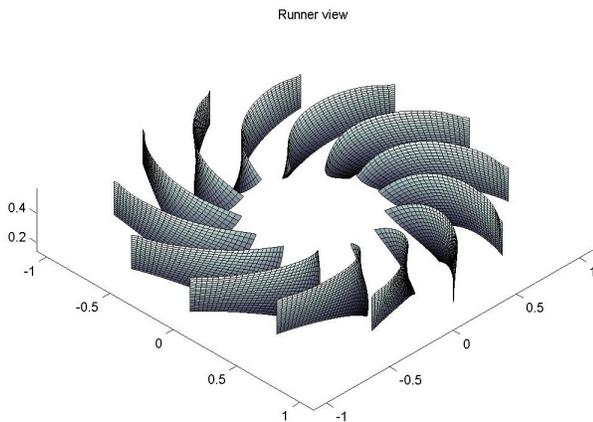
**Figure 10:** isometric view of runner blades
