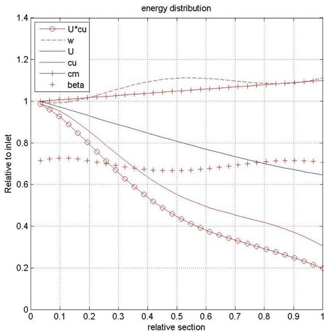
Figure 6: Energy distribution along streamline
