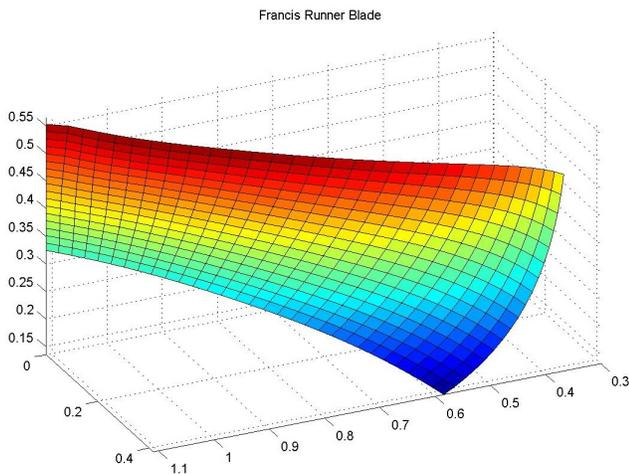
**Figure 9:** 3D plot of single blade
