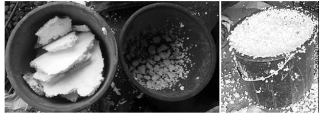
Figure 4: Segregation of EPS beads from used EPS boards
