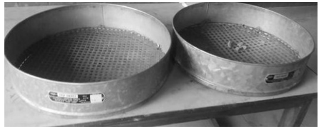
Figure 5: Sieves used to obtain aggregates of size range 10mm - 12.5mm
