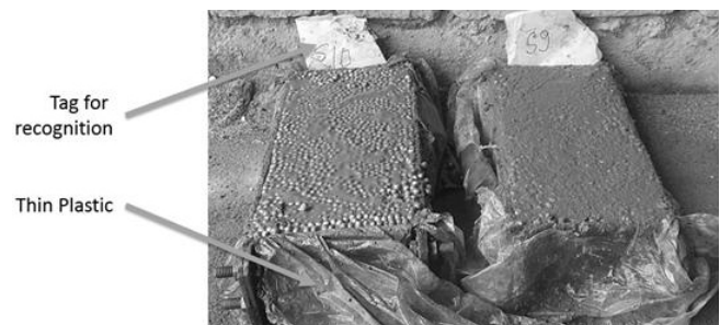
Figure 7: Placing the fresh concrete in the brick moulds
