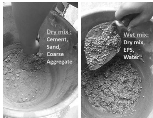
Figure 6: Dry mixing followed by wet mixing of the ingredients
