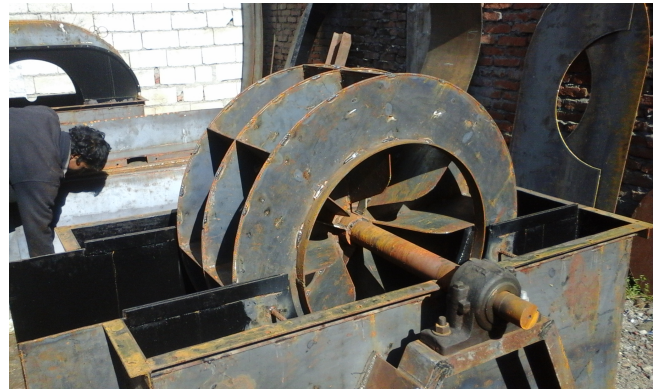
Figure 1: Centrifugal Blower used in Brick kiln
