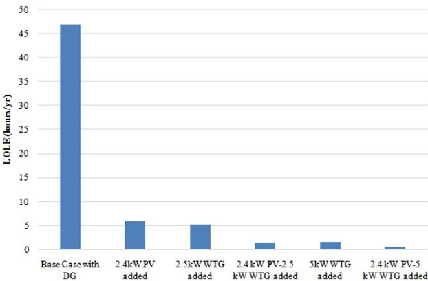
Figure 13: Effect of Renewable energy addition in DG system on LOLE
