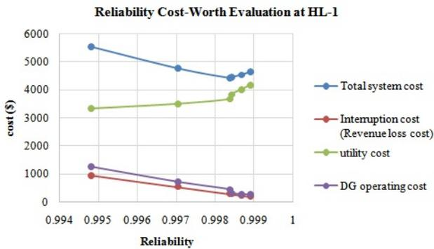
Figure 9: Reliability Cost component graph for PV-Battery-DG System
