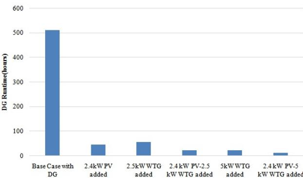
Figure 14: Effect of Renewable energy addition in DG system on DG runtime
