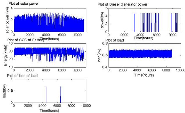
Figure 8: MATLAB output graph for PV-Battery-DG System
