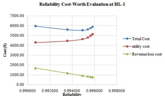
Figure 7: Reliability Cost Component graph for PV-Wind-Battery System
