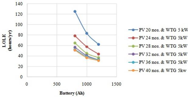
Figure 12: Effect of Battery Capacity in LOLE
