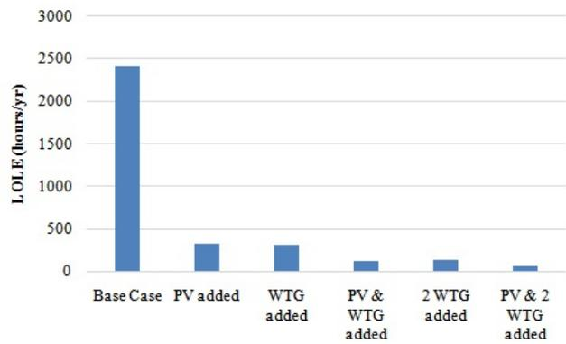
Figure 10: System risk with different energy sources added to the base system
