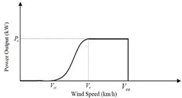
Figure 1: Wind Turbine Generator Power Curve
