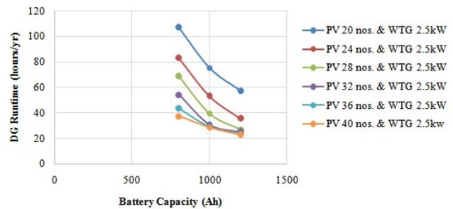
Figure 15: Effect of Battery capacity on DG runtime in PVBatteryDG System
