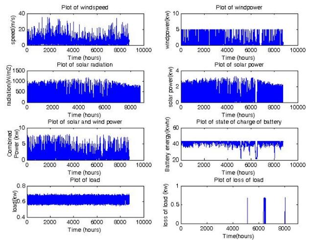
Figure 6: MATLAB output graph for PV-Wind-Battery System
