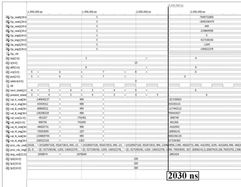
**Figure 7: Simulation Waveform from test of 16-point FFT**
