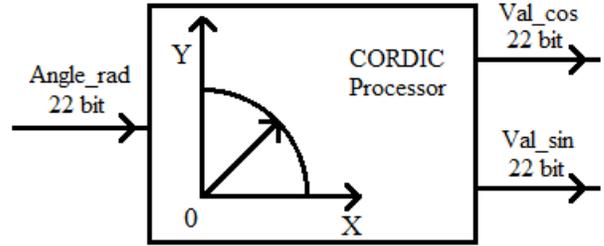
Figure 5: CORDIC Processor Block
