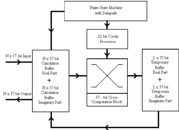
Figure 3: Block Diagram of Designed System
