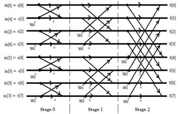
**Figure 1: Radix-2 Decimation in Time (DIT)-FFT algorithm for 8-points**
