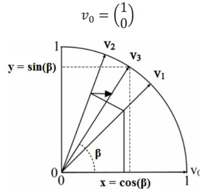
**Figure 2: Illustration of CORDIC Algorithm** (Wikipedia, 2014)
