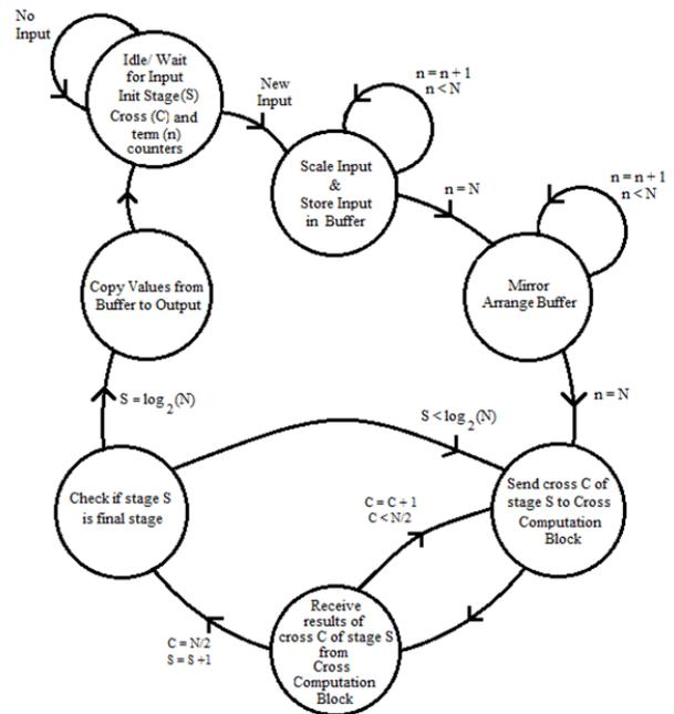
Figure 6: Schematic representation of the states of the FSMD
