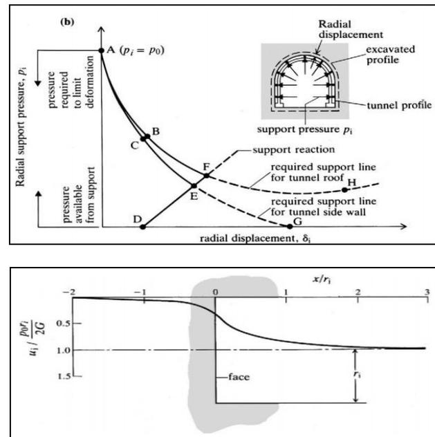
Figure 5: Distribution near the face, of the radial elastic displacement,  $u_i$ ,
