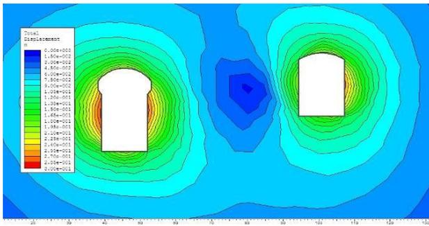
Figure 10: Plastic deformation contours
