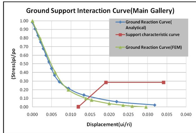
Figure 20: Ground Support Interaction Curve for the main gallery
