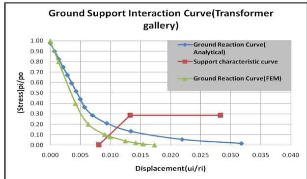
Figure 21: The Ground Support Interaction Curve for the Transformer Gallery
