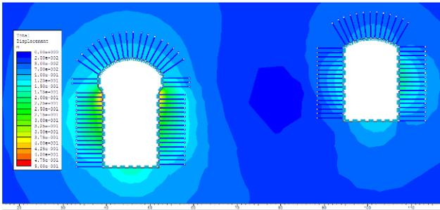
Figure 18: Total displacement after support installation
