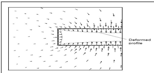
Figure 4: Sectional view of a three-dimensional finite element model of tunnel
