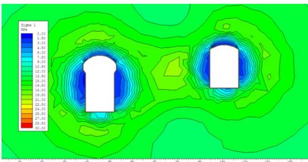
Figure 16: First Principle Stress (Plastic) around the two caverns in 2 dimensions (Phase2)
