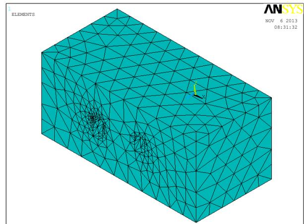
Figure 6: Mesh Generation in ANSYS
