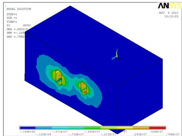
Figure 13: First Principle Stress around the two caverns in 3 dimensions (ANSYS)
