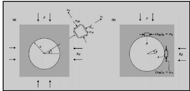
Figure.3: A circular excavation stress analysis in polar coordinate system for deducing the stress and displacement distribution around a circular excavation in a biaxial stress field
