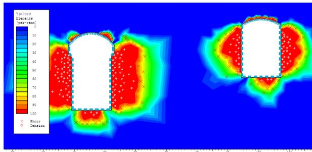
Figure 19: Confined yielded zone after support installation
