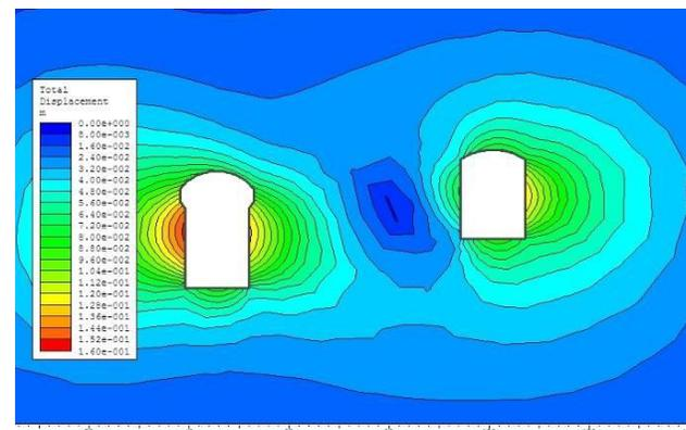
Figure 9: Elastic deformation contours
