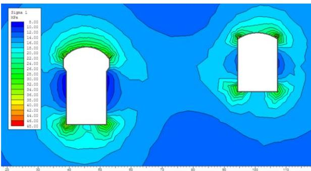
Figure 15: First Principle Stress (Elastic) around the two caverns in 2 dimensions (Phase2)
