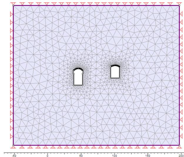
Figure 7: Mesh Generation in Phase2
