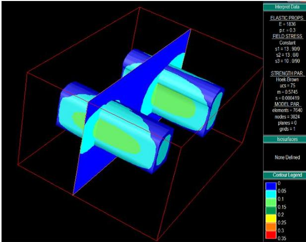
Figure 11: Elastic deformation contours from Examine 3D
