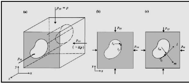
**Figure 1: An opening in a medium subject to initial stresses, for which is required the distribution of total stresses and excavation-induced displacements.**
