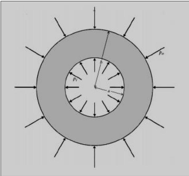
Figure 2: A thick-walled cylinder of elastic material, subject to interior pressure,  $p_i$ , and exterior pressure,  $p_o$
