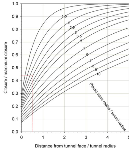
Figure 17: Vlachopoulos and Diederichs chart for determining tunnel closure before first installation of support
