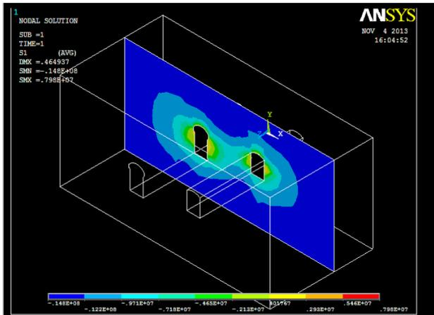
Figure 14: First Principle Stress around the two caverns sliced (ANSYS)
