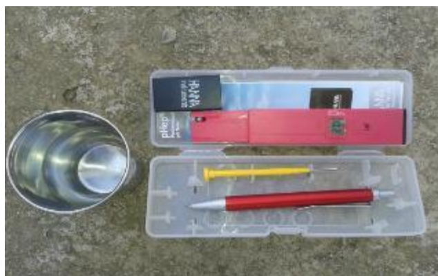
Figure 4: pH meter with buffer 7.0 solution for calibration
