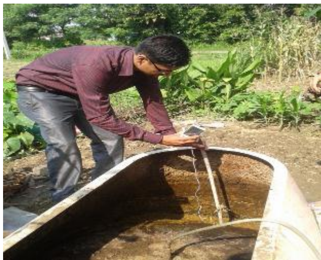
Figure 5: Measurement of inlet temperature of digester of FRP at Chitwan
