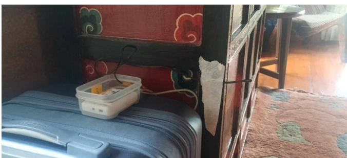
Figure 15: Measurement of internal temperature at 0.1m height
