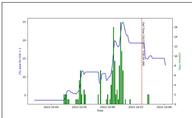
**Figure 3:** Percentage Area of Failure and Rainfall event at various times
