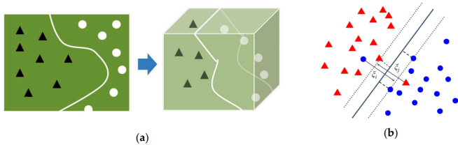
Figure 4: Explanation of SVM principle. (a) optimum n – dimensional Hyperplane differentiating binary datasets with maximum gap (b) non - separable case and slack variables \xi_i [7, 27]
